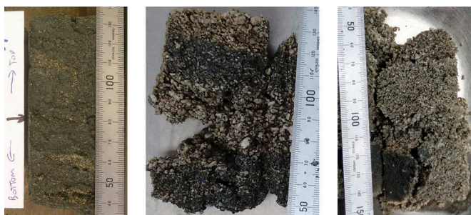
Figure 6. View of inside of triaxial specimens. Left: 3-GPS1 A (Low pumice content). Middle: 3-GPTR3 A (Medium-high pumice content). Right: 3-GPTR2 B (High pumice content)
