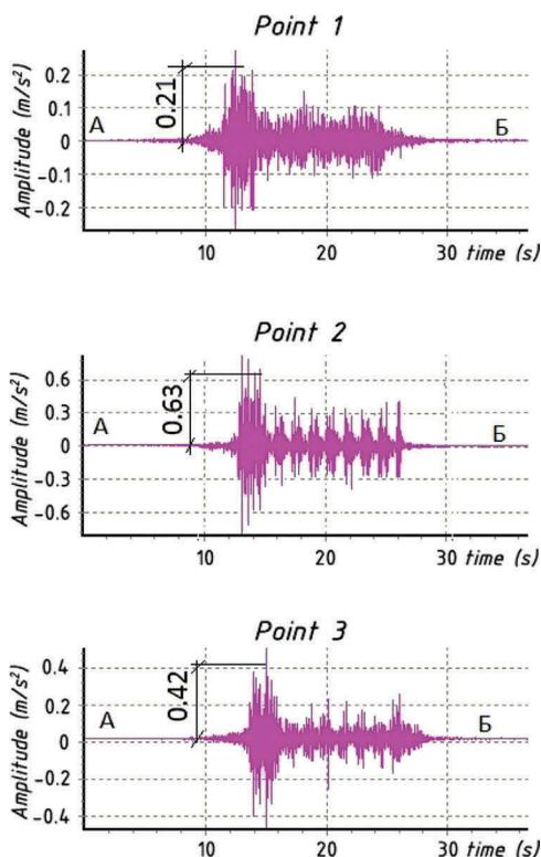
Figure 7. Time signal of the PS horizontal vibration accelerations (X direction) in case of passengers train moving from point 1 to point 3 (Figure 6).
