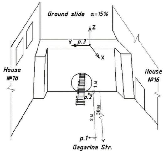
Figure 2. Location of vibration sensors in point 1, point 2 and point 3 for researches performance.
