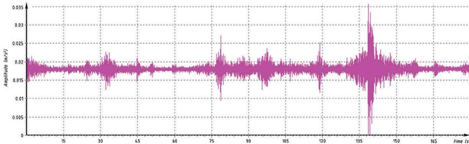
Figure 3. Z in point 3 retaining wall vibrations accelerating graphics.
