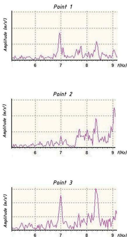
Figure 8. Amplitude spectrum of the PS horizontal vibration accelerations (X direction) in case of passengers train moving from point 1 to point 3 (Figure 6).
