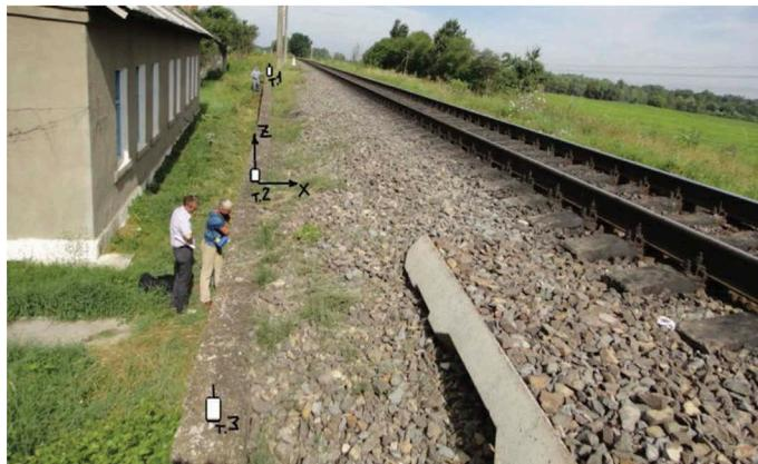
Figure 6. Location of vibration sensors during retaining wall investigation.
