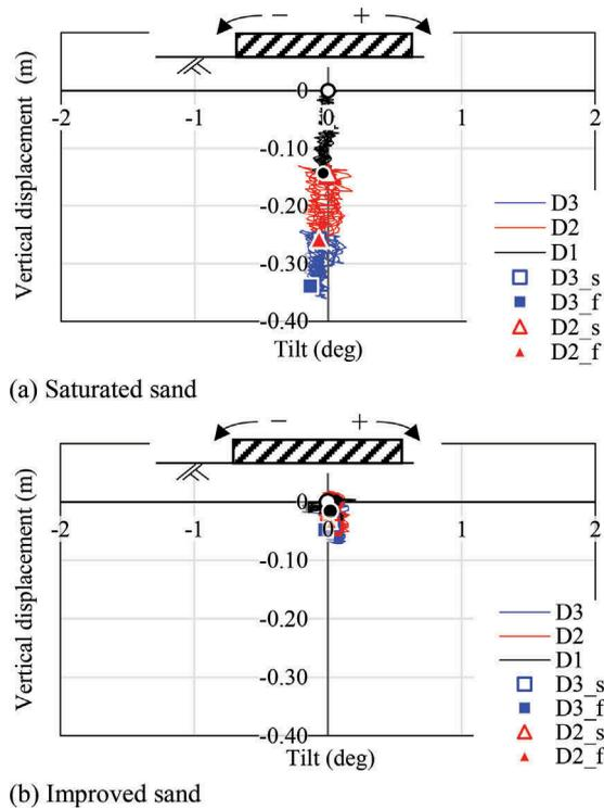
Figure 11. Relationships between tilt and Vertical displacement
