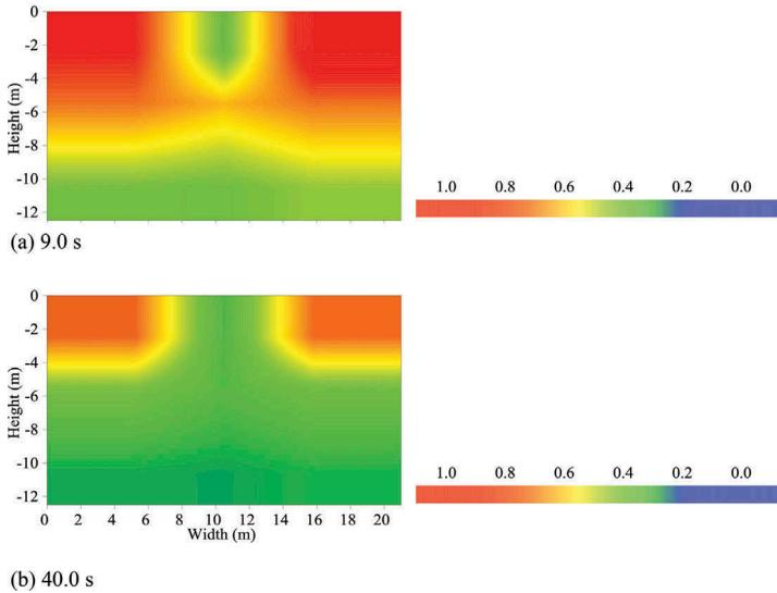
Figure 6. EPWP ratio on Saturated sand
