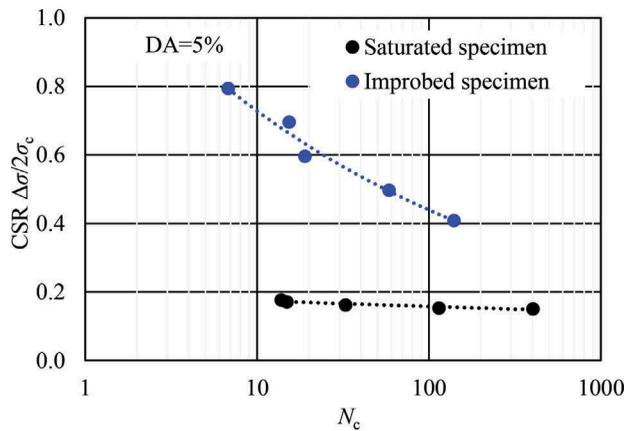
Figure 2. Liquefaction resistance
