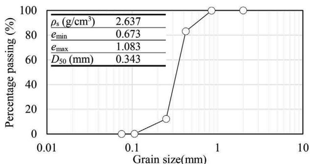
Figure 1. Grain size of silica sand No 6
