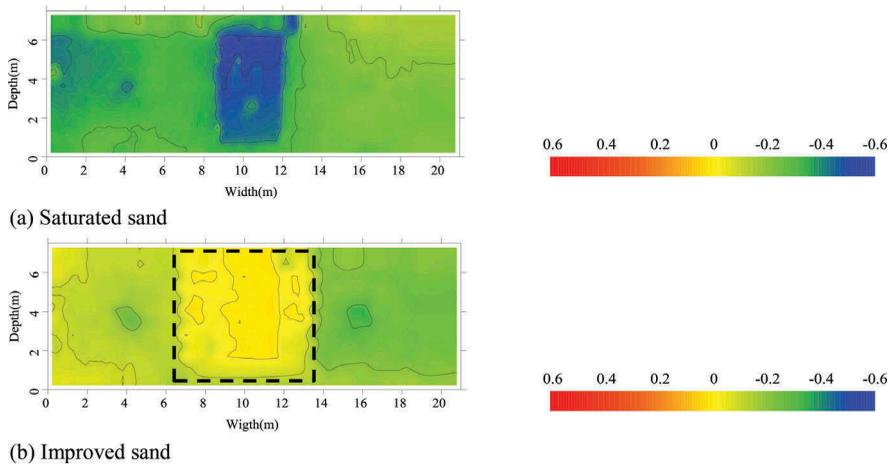
Figure 9. Surface displacement before and after shakings
