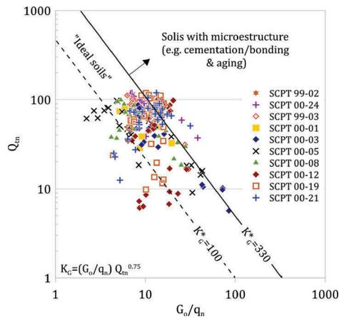
Figure 6. Correlation between normalized cone tip resistance and small strain shear modulus measured in seismic cone tests for the Mission Bridge site.
