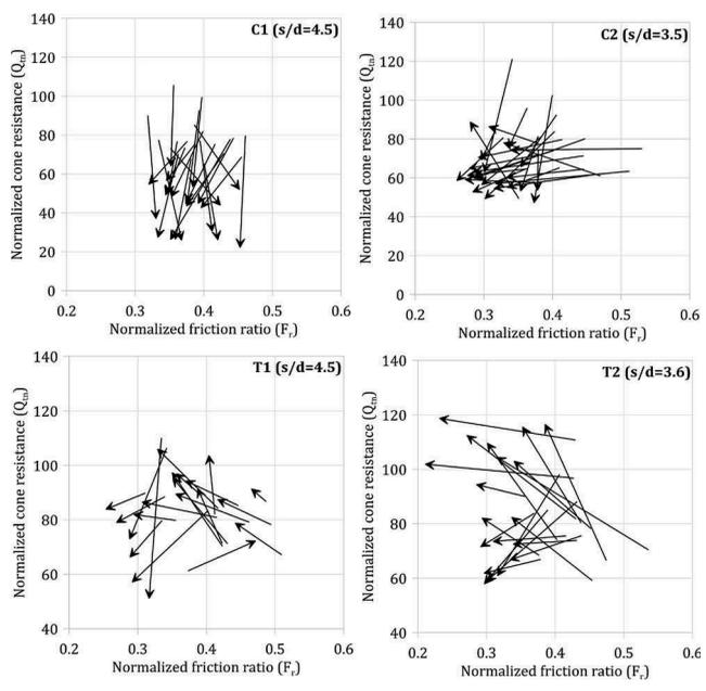
Figure 5. Evaluation of ground improvement based on normalized cone resistance and normalized friction ratio.
