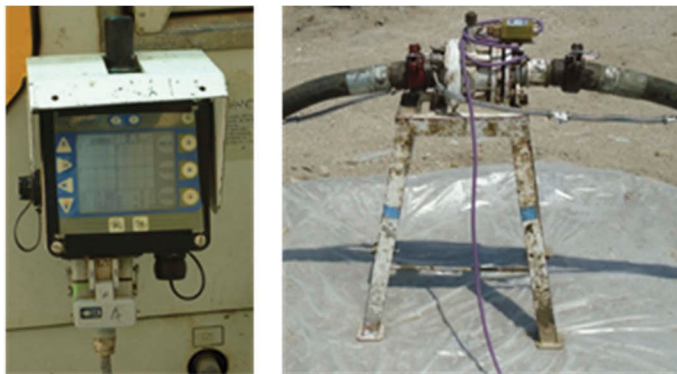
Figure 11. Automated data acquisition and processing system and pressure sensor.
