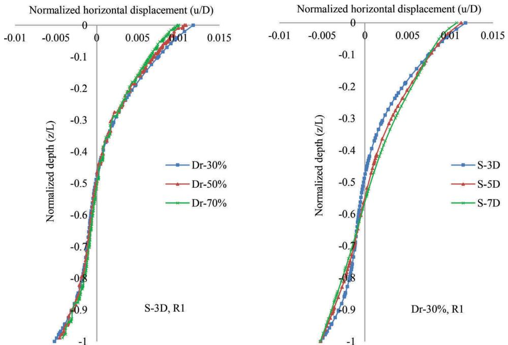
Figure 2. Normalized lateral pile displacement for varying (a) Relative densities and (b) Pile spacing
