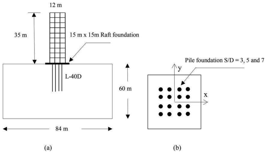
Figure 1. (a) Elevation and (b) Plan view of 4 x 4 Pile foundation arrangement
