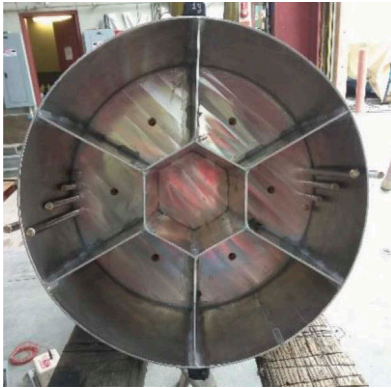
Figure 1. Bottom view of the suction caisson showing the honey-comb shaped compartments.
