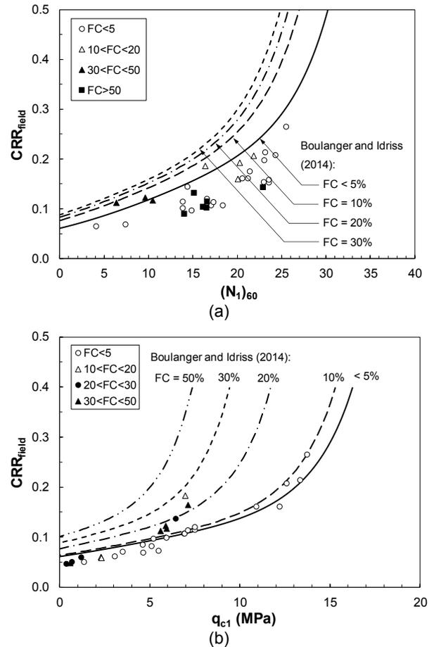
Figure 3. Comparisons of corrected (a) CRR- $(N_1)_{60}$ , and (b) CRR- $q_{c1}$  data collected in this study with liquefaction triggering boundaries established from case histories of liquefaction occurrence (Boulanger and Idriss 2014).
