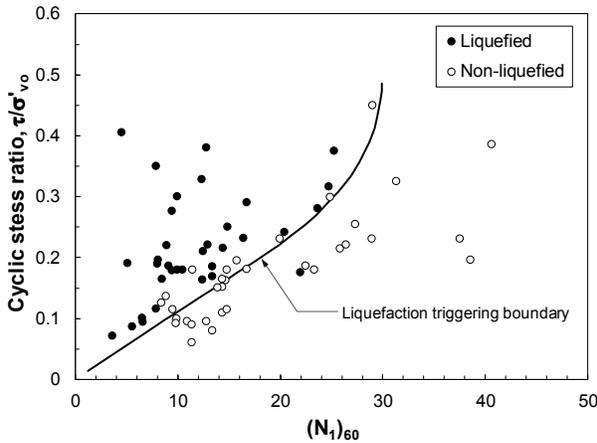
Figure 1. Liquefaction assessment chart of Seed et al. (1985) for  $M = 7.5$  earthquakes,  $\sigma'_{vo} = 100$  kPa, and  $FC \leq 5\%$
