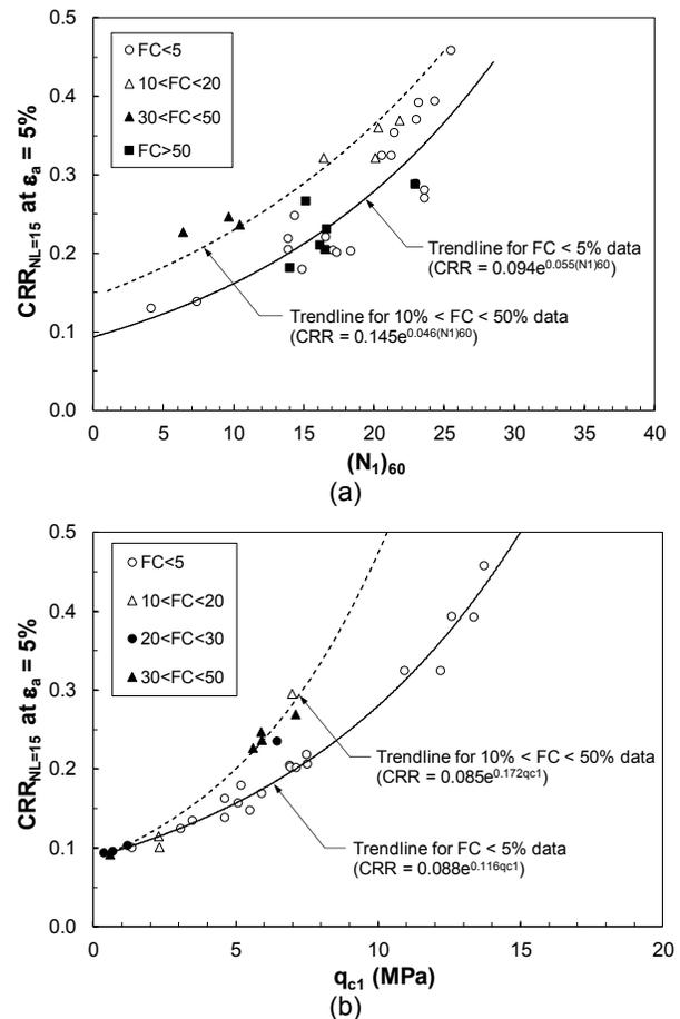
Figure 2. Plots of cyclic resistance ratio for liquefaction triggering in 15 uniform cycles from the cyclic triaxial tests of Tables 1 and 2 versus (a)  $(N_1)_{60}$ , and (b)  $q_{c1}$
