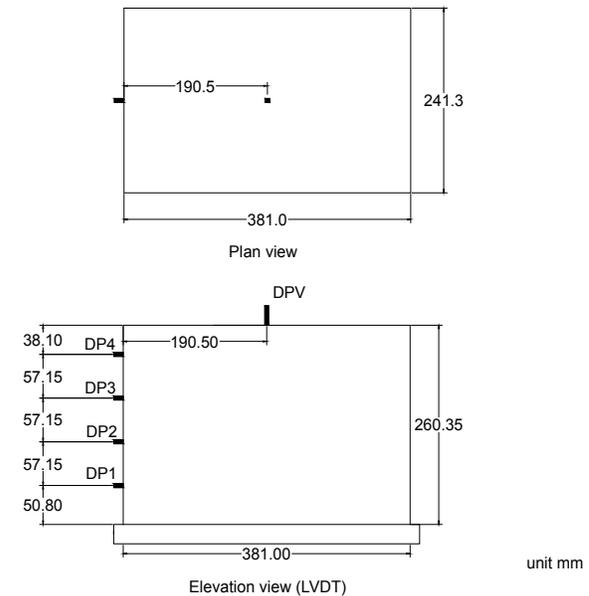
Figure 5. Location of LVDTs for centrifuge testing
