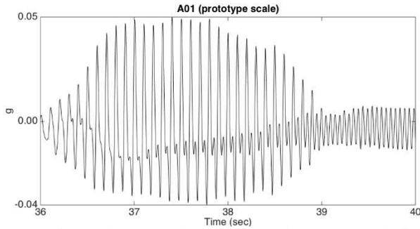
Figure 6. Input acceleration at the container base at 10g
