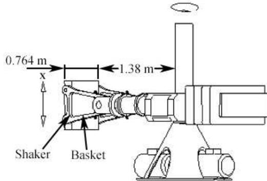
Figure 3. Direction of shaking on the ES-9 shaker
