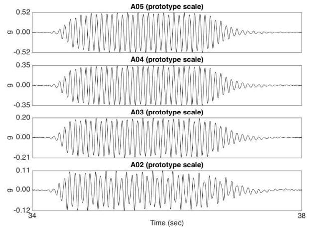
Figure 10. Results from accelerometers along the container laminates at 30 g
