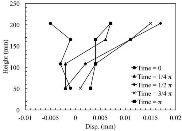
Figure 17. Displacements at different depths in the soil layer at 10 g test along the container.
