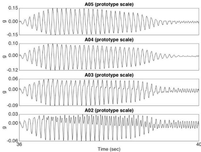
Figure 7. Results from accelerometers along the container laminates at 10 g
