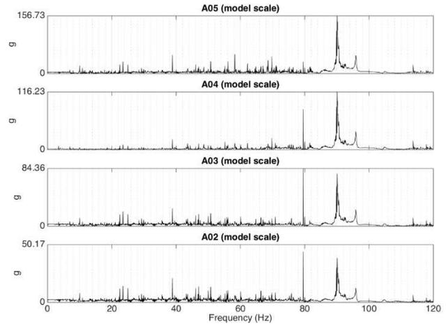
Figure 19. Accelerations at model scale with frequency domain from the 10 g test
