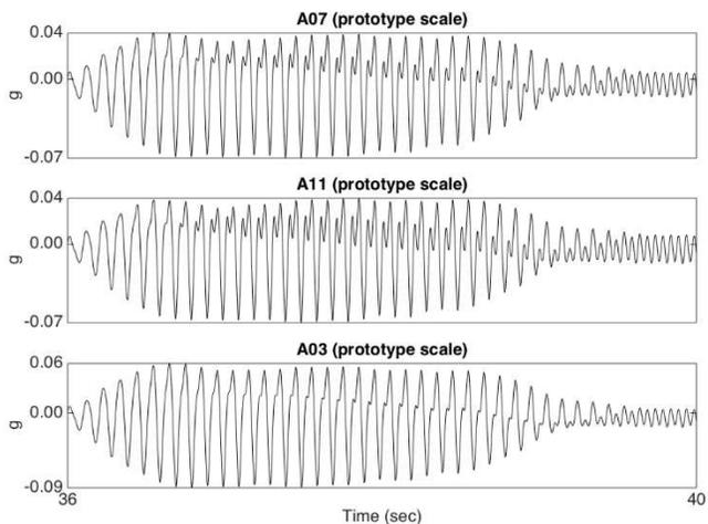
Figure 8. Results from accelerometers at same height (107.95 mm from the base) at 10 g
