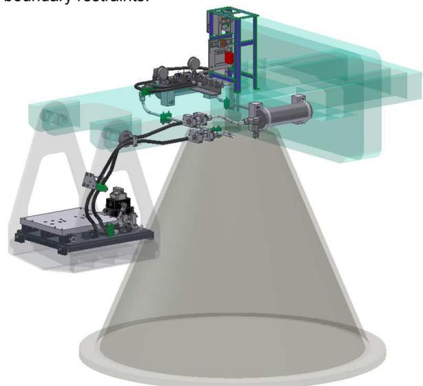
Figure 2. UCSD centrifuge shaker system
