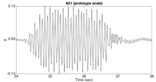
Figure 9. Input acceleration applied to the base at 30 g
