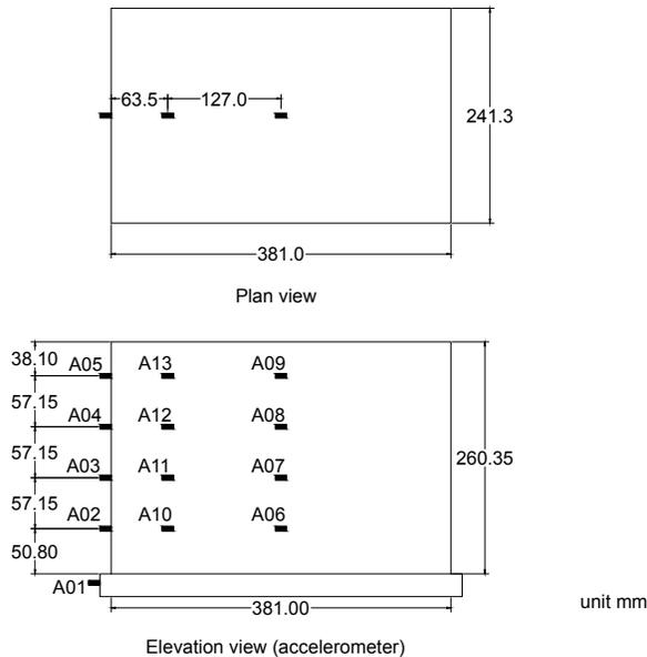
Figure 4. Location of accelerometers for centrifuge test
