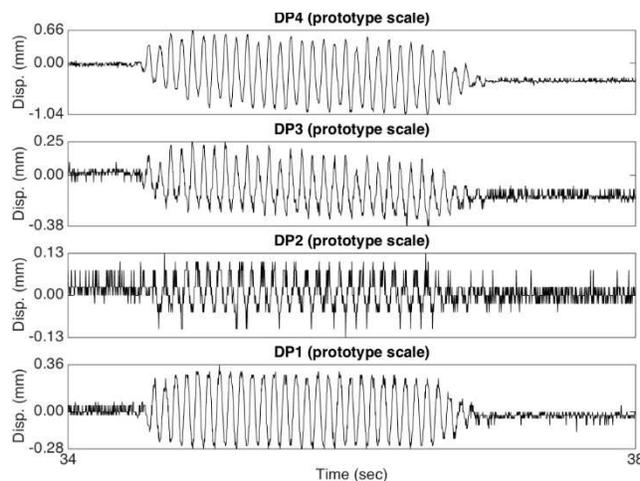
Figure 13. Horizontal displacement of each laminate
