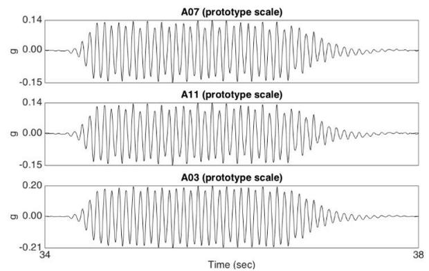
Figure 11. Results from accelerometers at the same height (107.95 mm from the base) at 30 g
