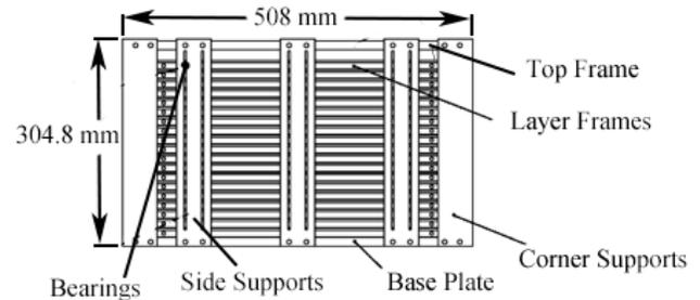
Figure 1. Dimensions and components of the laminar container
