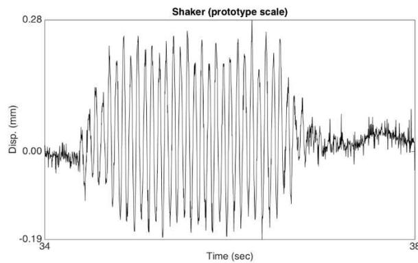
Figure 12. Horizontal displacement of the shaker
