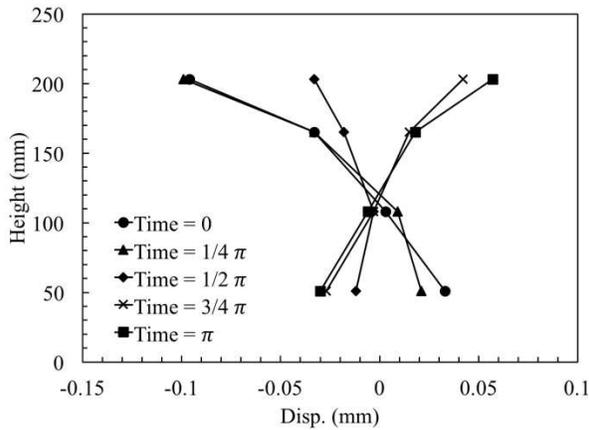
Figure 18. Displacements at different depths in the soil layer at 30 g test located along the container.
