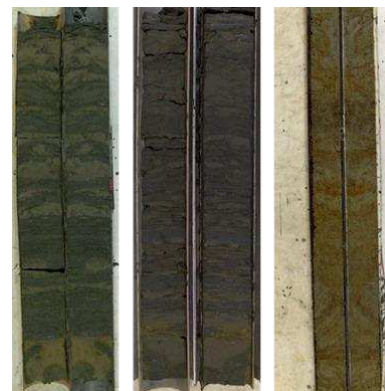
Figure 1. Tubes of laminated deposits with alternating thin layers of sand and clay.
