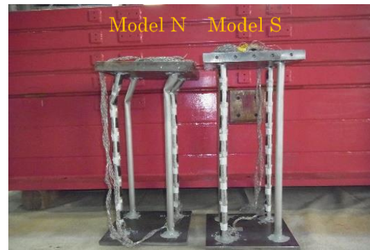
Photo 1. Structure model after large shaking
