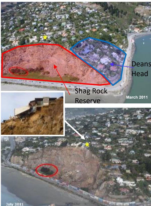
Figure 3. Shag Rock Reserve photographs taken in March 2011 and July 2011. Note the row of double stacked shipping containers protecting the road from rockfall
