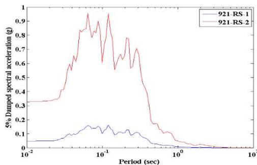
Figure 2. Damped spectral acceleration of input motions
