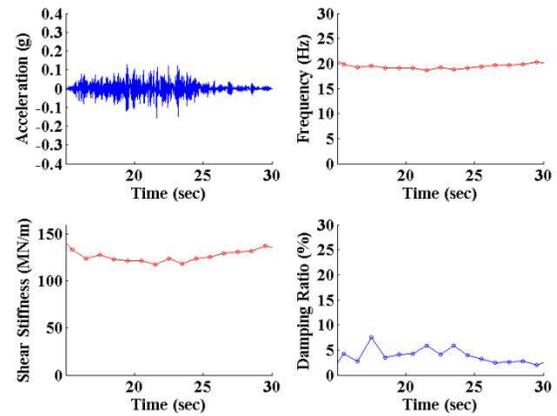
Figure 11. Short time system identification for soil in Case 921-RS-1
