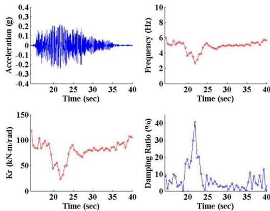
Figure 10. Short time system identification for structure in Case 921-RS-2
