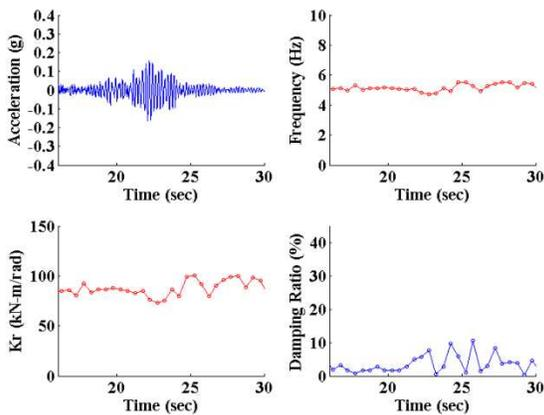
Figure 9. Short time system identification for structure in Case 921-RS-1
