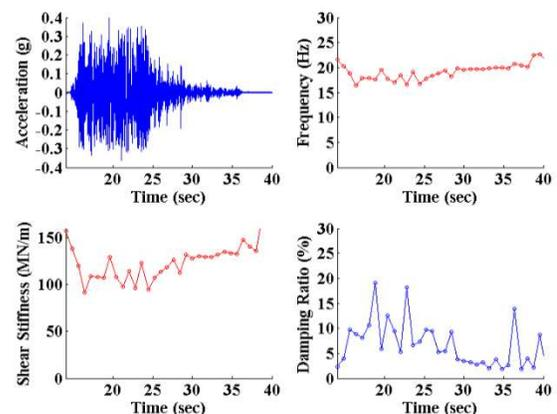
Figure 12. Short time system identification for soil in Case 921-RS-2
