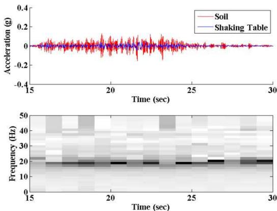
Figure 7. Short time transfer function for soil in Case 921-RS-1
