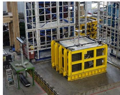
Figure 1. Arrangement of shaking table testing (from Chiou et al. 2014)
