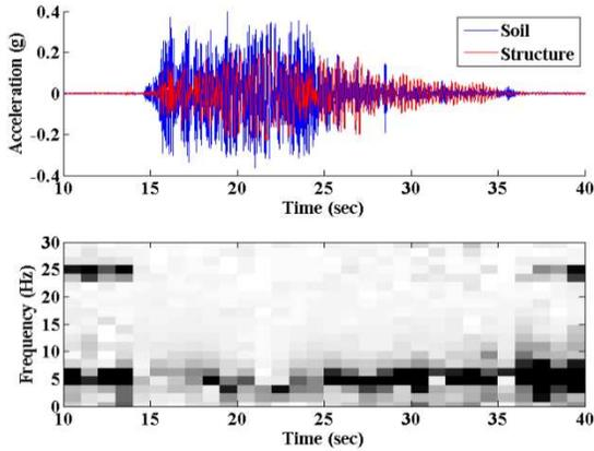
Figure 6. Short time transfer function for structure in Case 921-RS-2
