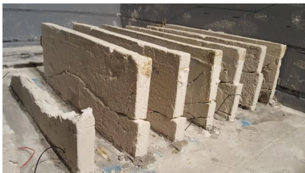
Figure 12. Post-test excavation photo of the soil-cement walls (toe of berm is on left side of photograph)
