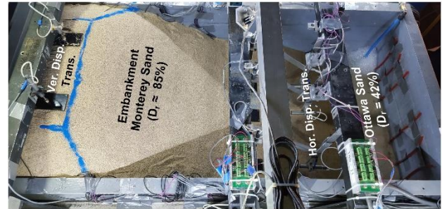
Figure 4. Embankment model after completion
