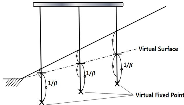
Figure 1. Determining the virtual fixed point
