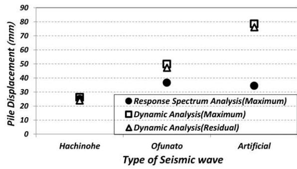
(b) Comparison of pile displacement
