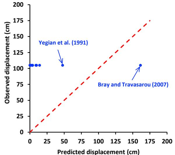
Figure 8. Observed vs. predicted displacements of Zipingpu dam obtained from simplified models.
