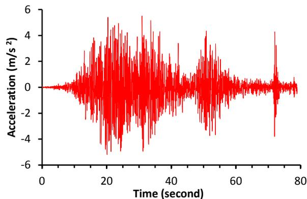
Figure 5. Acceleration time history of the "5.12" earthquake (scaled to 0.55g).
