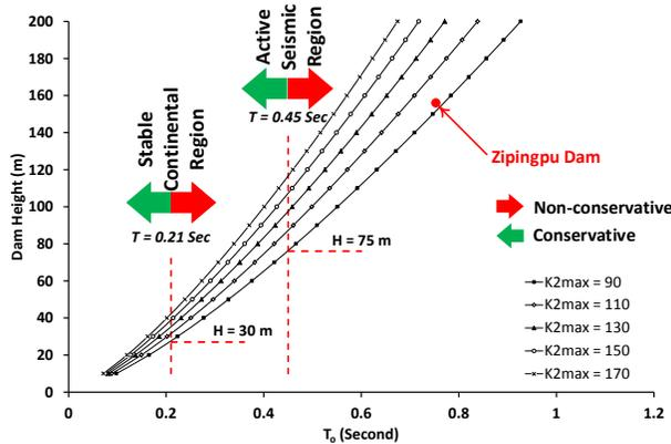
Figure 3. Variation of fundamental period with height for rockfill dams.
