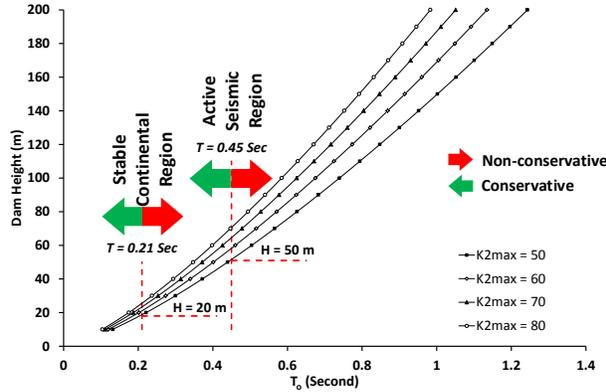
Figure 2. Variation of fundamental period with height for earthfill dams.
