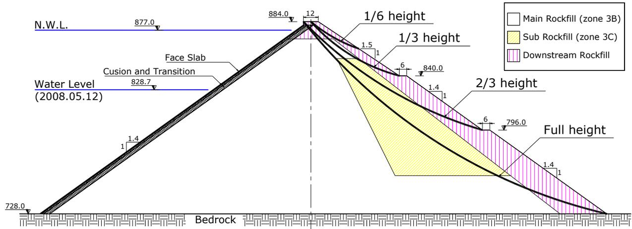
Figure 4. Deepest cross section of Zipingpu dam (cross section 0+251, all units in Meters) and location of slip surfaces.
