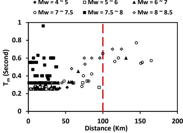
Figure 1. Variation of the period of earthquakes versus distance in 152 dams (data from Singh and Roy, 2009).
