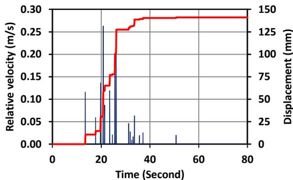
Figure 7. Records of relative velocity (blue) and permanent displacement (red) of the shallowest sliding block.
