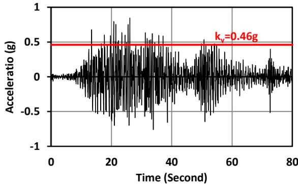
Figure 6. Acceleration time history for the shallowest sliding block in Zipingpu dam.
