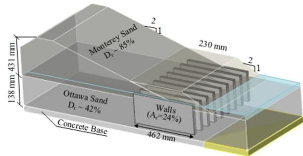
Figure 2. Centrifuge model configuration with dimensions in model scale
