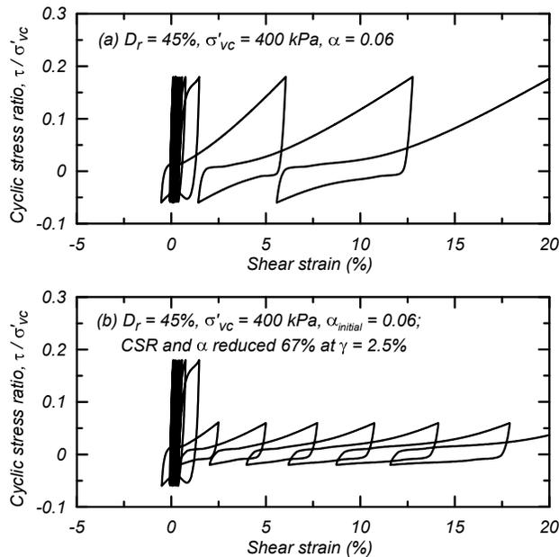
Figure 9. Response of calibrated PM4Sand model in cyclic undrained simple shear loading with an initial static shear stress ratio of  $\alpha = 0.06$ : (a) with a uniform applied CSR, and (b) with the CSR and  $\alpha$  reduced 67% once the peak shear strain reached 2.5%
