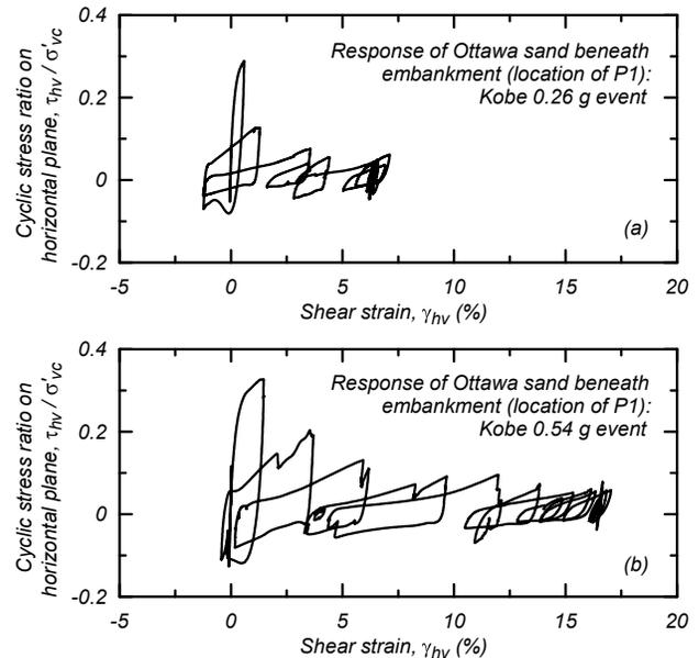
Figure 15. Stress-strain response for a point in the loose Ottawa layer beneath the embankment crest (location of P1) during: (a) Kobe 0.26 g and (b) Kobe 0.54 g events
