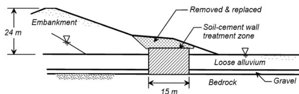
Figure 1. Soil-cement shear walls at Clemson Diversion Dams, SC (after Wooten and Foreman 2005)
