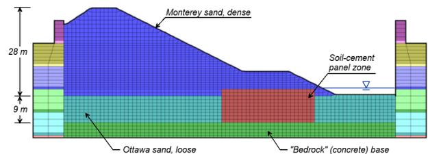
Figure 7. Two-dimensional mesh and material zones
