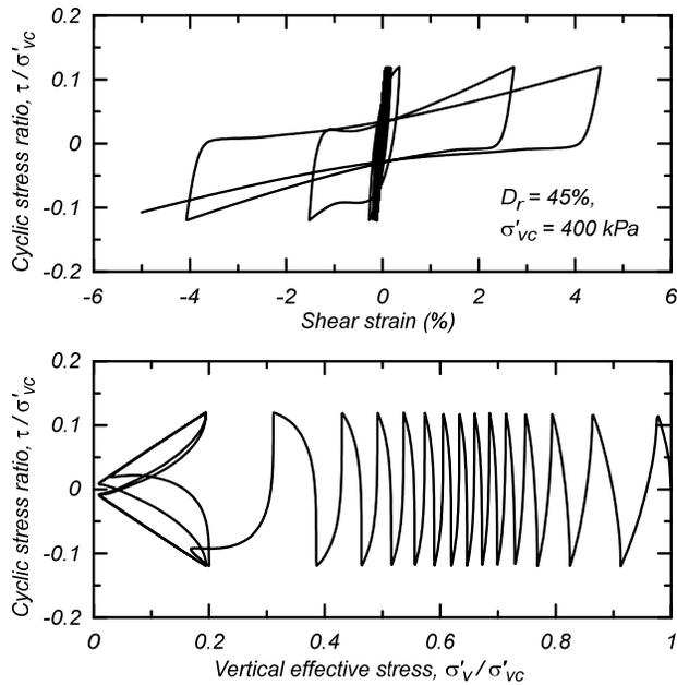
Figure 8. Response of calibrated PM4Sand model in cyclic undrained simple shear loading with zero initial static shear stress
