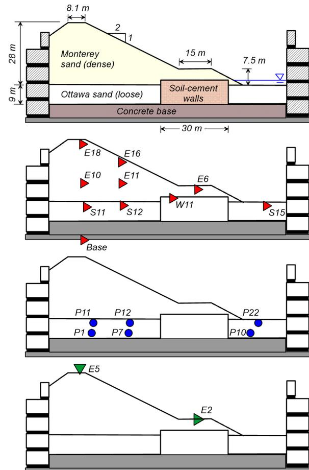
Figure 3. Cross-sections showing model dimensions (prototype scale) and the locations of accelerometers (red triangles), pore pressure transducers (blue circles), and displacement transducers (green triangles) that are later compared with simulation results
