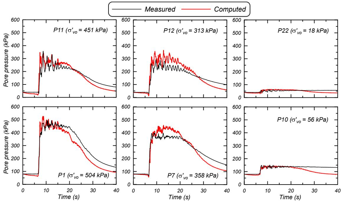
Figure 12. Measured and computed excess pore water pressures for the Kobe 0.26 g event
