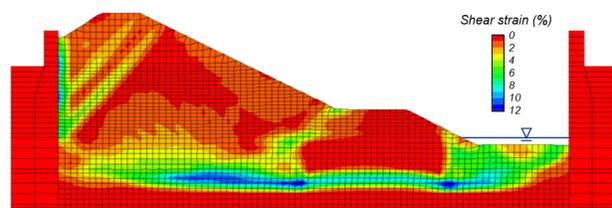
Figure 14. Contours of shear strain after shaking for the simulation of the Kobe 0.26 g event
