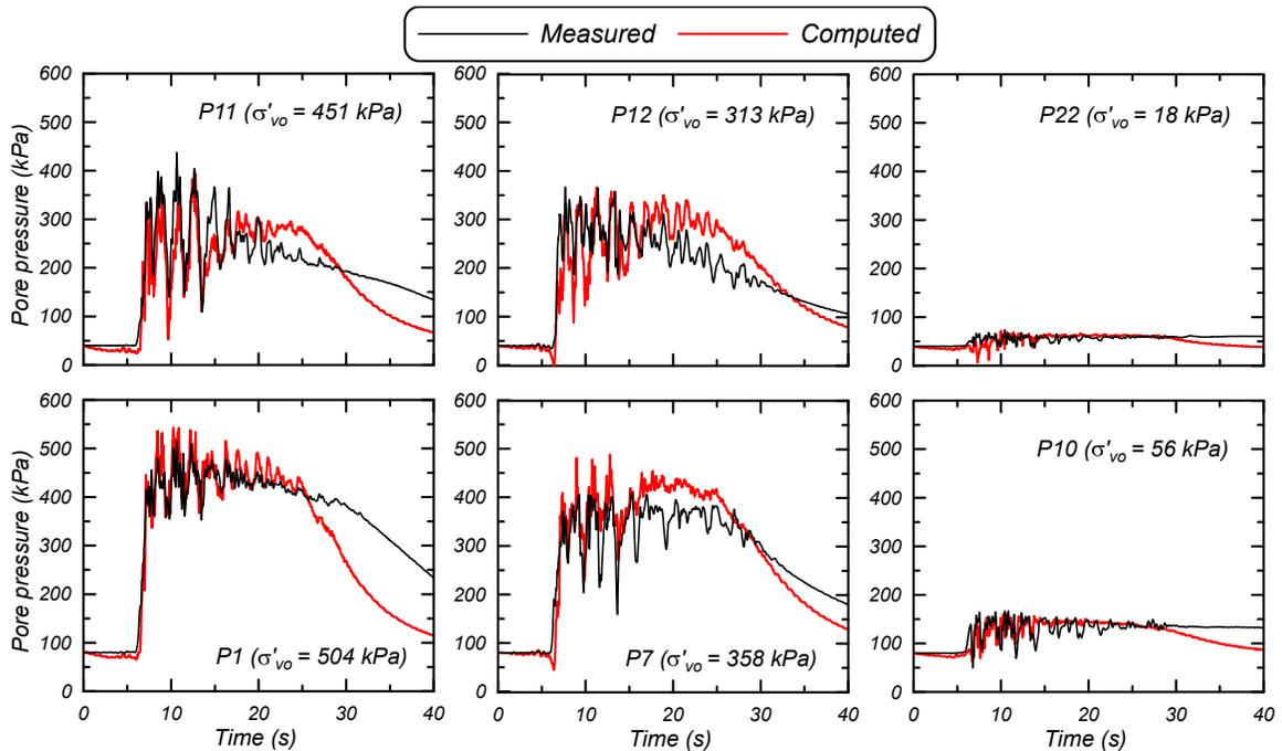
Figure 17. Measured and computed excess pore water pressures for the Kobe 0.54 g event
