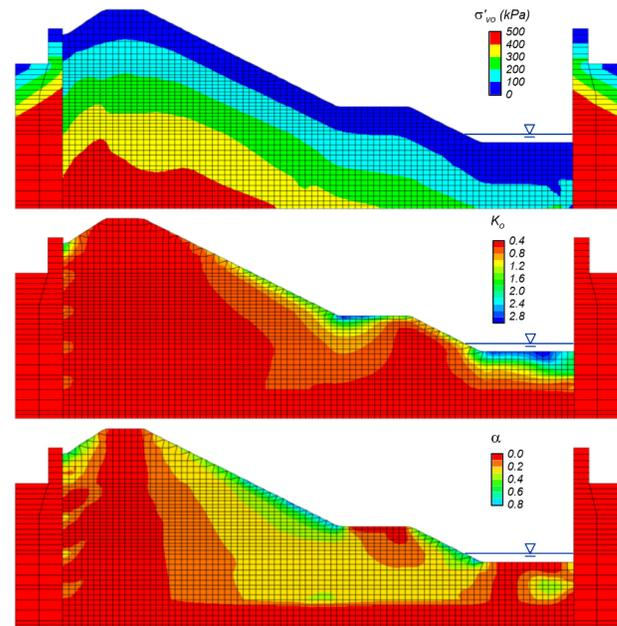
Figure 10. Initial static stress conditions: vertical effective stress, coefficient of lateral earth pressure at rest, and initial static shear stress ratio on horizontal planes.
