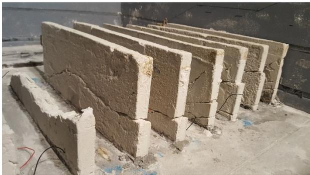
Figure 5. Post-test excavation photos of the soil-cement panels (toe of berm is to left side of photos)
