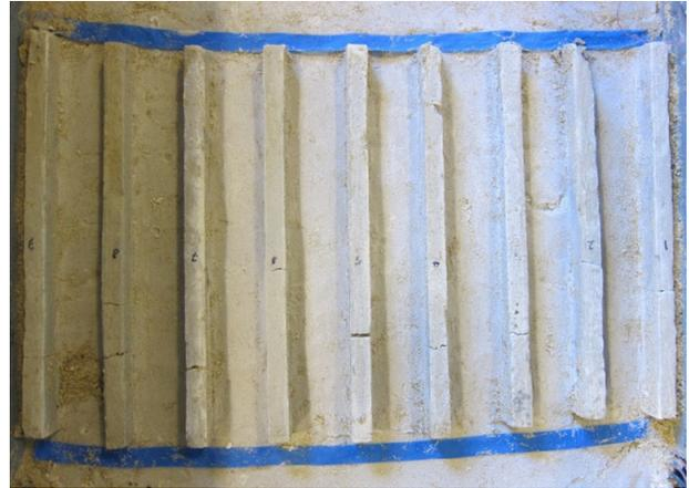
Figure 6. Post-test excavation with exposed paper markers (originally aligned in contact with panels) showing the liquefied sand moved more than the soil-cement panels (toe of berm is to bottom of photo)
