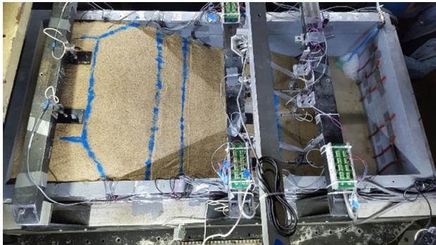
Figure 4. Photograph of model mounted on the centrifuge; lines of blue sand are for visual reference
