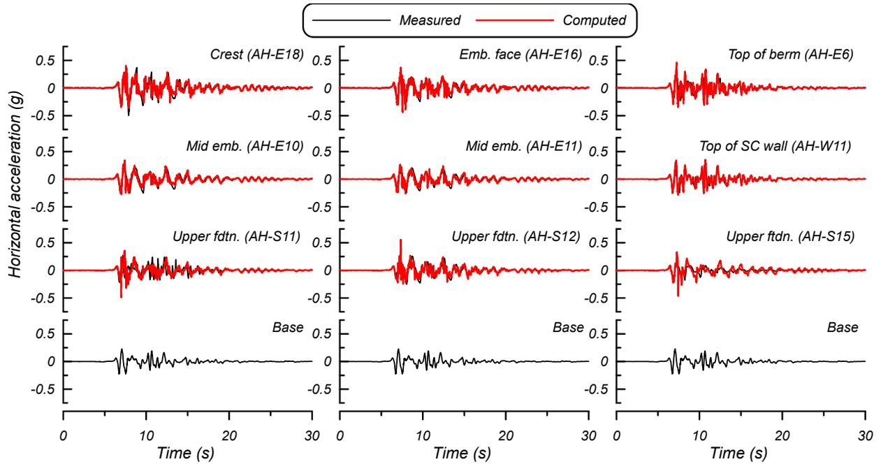
Figure 11. Measured and computed accelerations for the Kobe 0.26 g event
