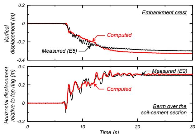
Figure 13. Measured and computed crest settlement and berm horizontal displacement for the Kobe 0.26 g event
