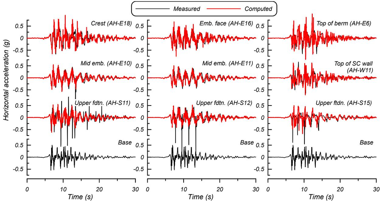
Figure 16. Measured and computed accelerations for the Kobe 0.54 g event
