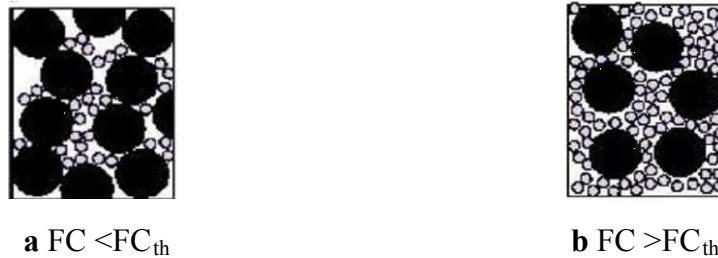
Figure 4. Schematic diagrams representing sand-silt mixtures: (a) Coarse grains are in contact with each other, (b) coarse grains are swimming in the fines matrix
