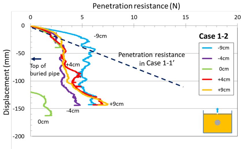
Figure 9. Penetration resistance after the test (Case 1-2)
