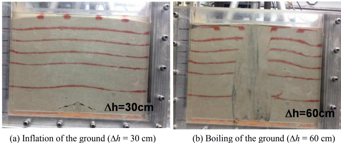
Figure 7. Boiling of the ground without pavement (Case 1-5).
