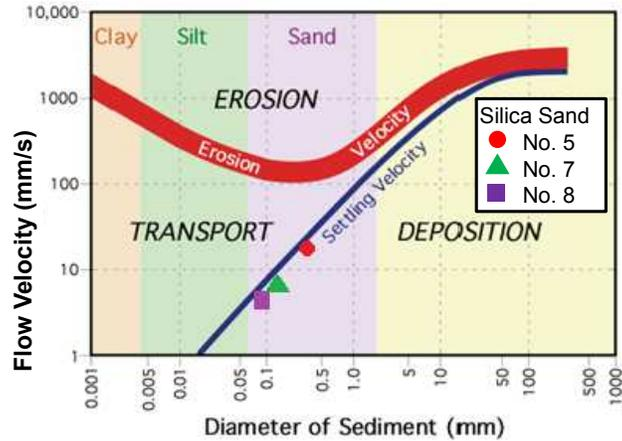
Figure 5. Relationship between grain diameter and flow velocity to start sand eruption (modified Pidwirny, 2006).
