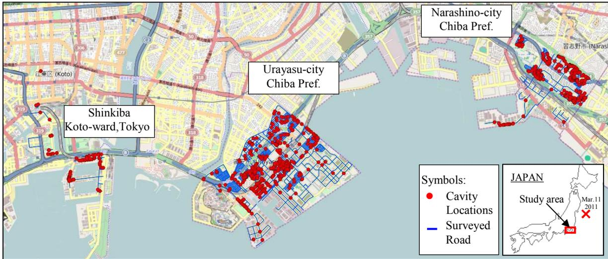
Figure 1. Locations of subsurface cavities caused by ground liquefaction.
