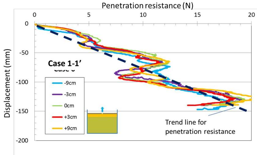
Figure 8. Penetration resistance after the test (Case 1-1')
