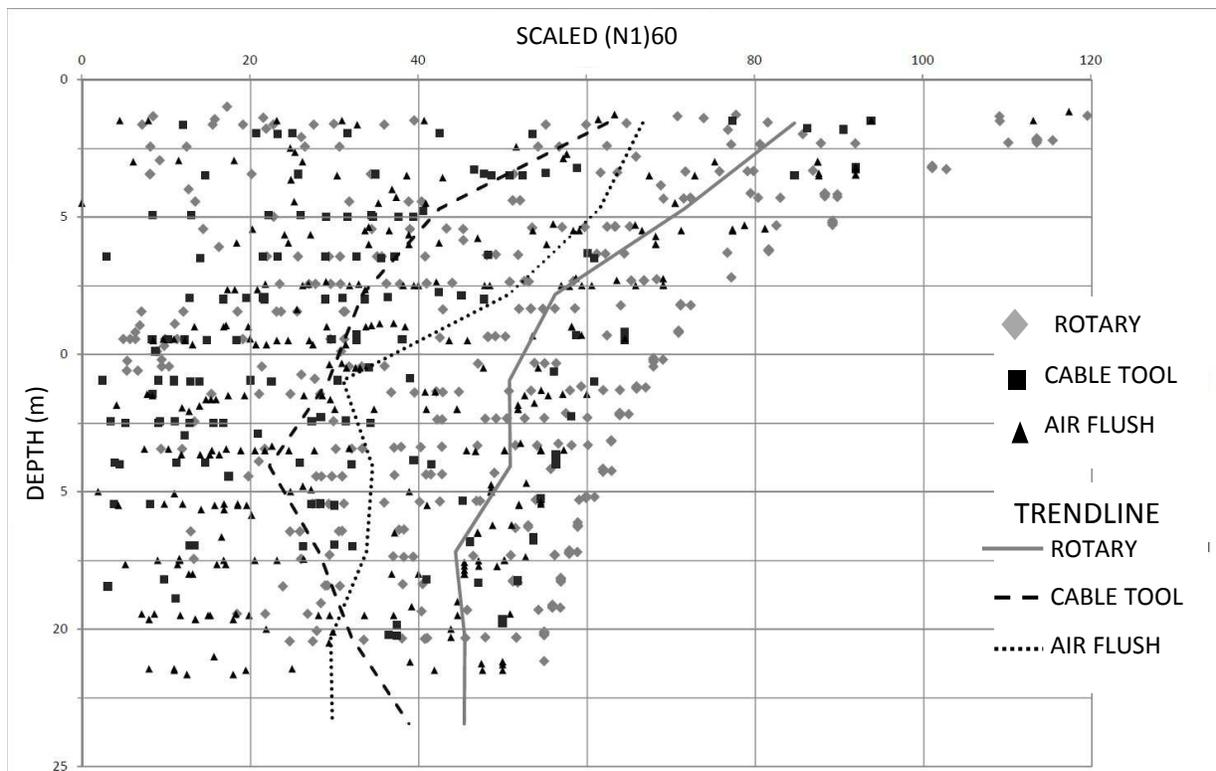
Figure 2: (N1)60 vs Depth for All Tests
