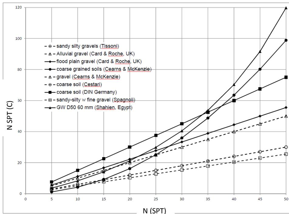
Figure 3: Correlations between SPT N and SPT N(C)
