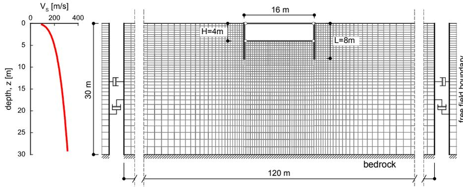
Figure 2. Model geometry and mesh for 2D analyses.
