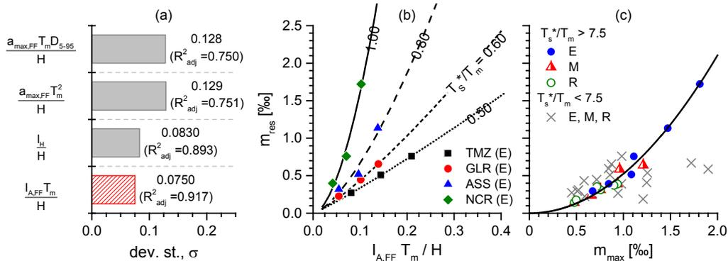
Figure 6. Standard error,  $\sigma$ , of data regression for different dimensionless IM parameters (a). Normalized residual bending moment,  $m_{res}$ , vs normalized Arias intensity condition and period ratio for natural records (E) ( $n_{eq} > 10$ ) (b). Normalized residual vs maximum moment (c).
