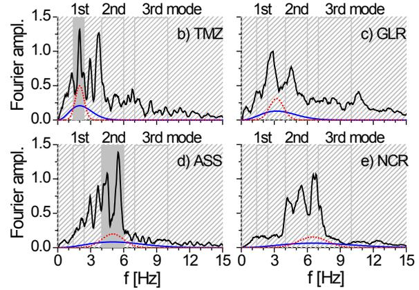
Figure 1. List of acceleration time history S01 (a) and seismic signals in frequency domain (b, c, d and e) of waveforms used in this study.
