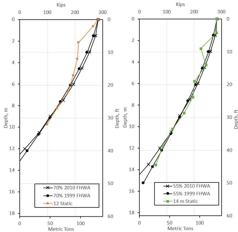
Figure 4. Interpreted pile load versus depth curves from static load tests in comparison with curves as a percentage of load predicted by 1999 and 2010 FHWA equations for drilled shaft design.
