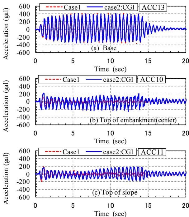
Figure 6. Response acceleration of base and embankment
