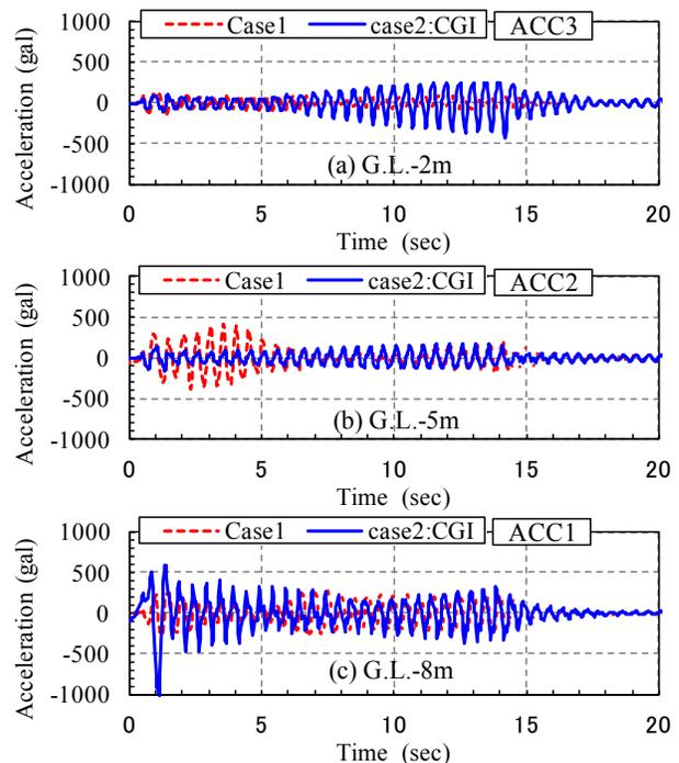
Figure 7. Response acceleration of sand layer (liquefaction layer)
