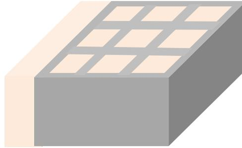
Figure 1. Image of latticed shaped ground improvement
