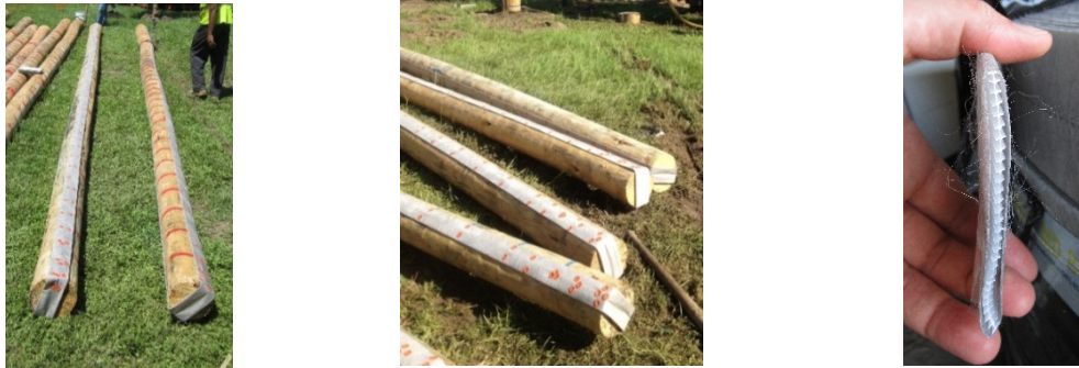
Figure 2. Drained timber piles and PVDs used in this study
