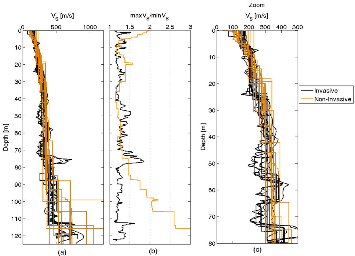
Figure 2 –Mirandola site: a) Shear wave velocity profiles from invasive (black) and non-invasive tests; b) ratio between the maximum and the minimum values of shear wave velocity for each population; c) close-up view of (a).
