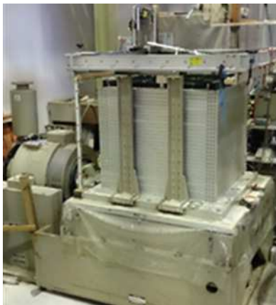
Figure 1. Laminar box and shaking table
