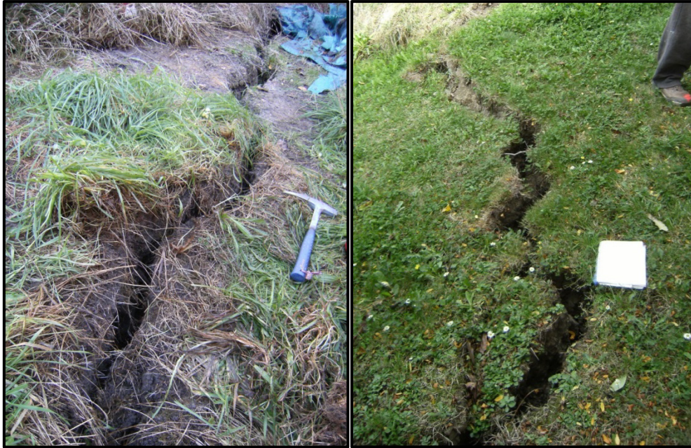
Figure 3: Ground fissuring at number 40 Rapaki Road (left) and number 3 Glenview Terrace (right). Both photographs taken facing south towards the head of the valley. Geological hammer and A4-size paper for scale.
