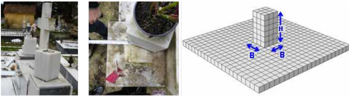
Figure 3. A marble vase observed in field (photos), modeled as rigid block on top of rigid base.
