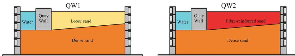
Figure 1 Centrifuge test layouts
