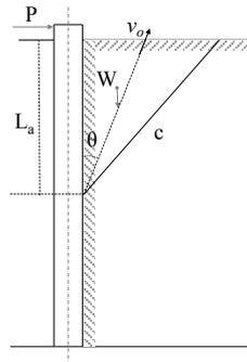
Figure 8. Soil Deformation Mechanism
