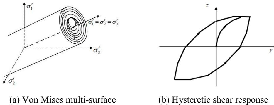
Figure 2. Von Mises multi surface kinematic plasticity model (after Lu et. al. 2006)
