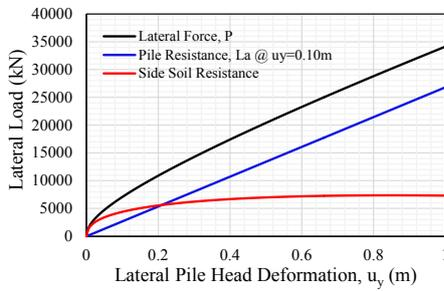
Figure 6. Load deformation curve
