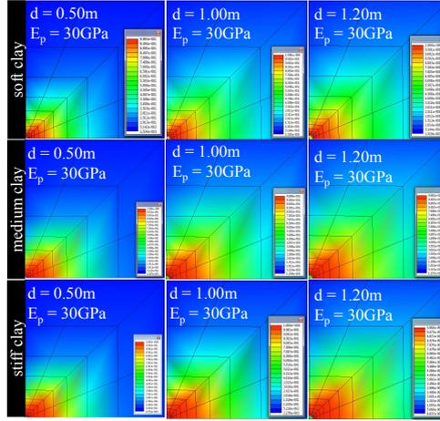
Figure 9. Stress ratio distribution for piles with diameter,  $d=0.5$ ,  $1.0$  and  $1.2\text{m}$  embedded in soft, medium and stiff clay in XY plane (top view)
