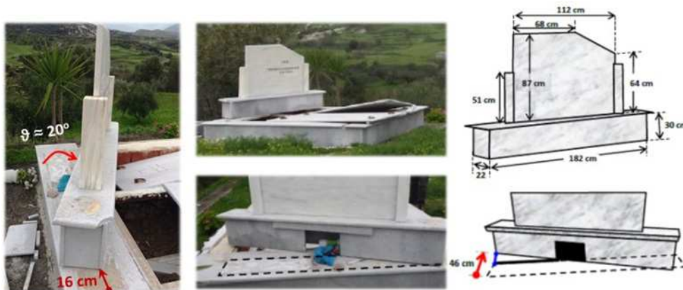
Figure 9. Photos and sketches with dimensions and displacement of a rotated headstone.
