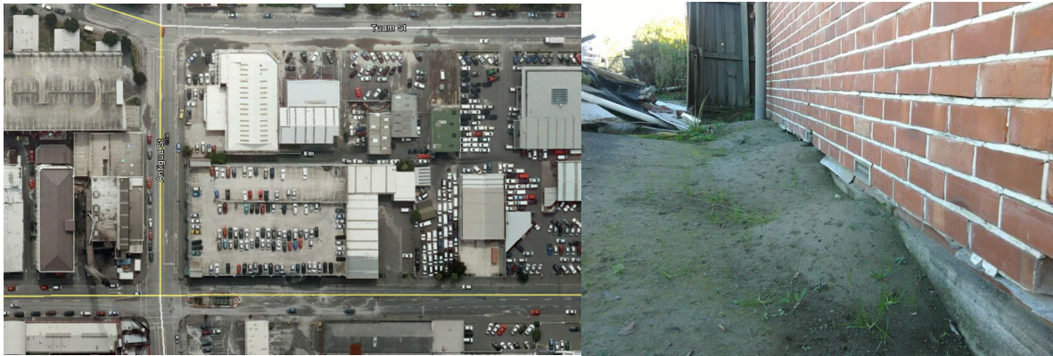
Figure 2. Liquefaction surface manifestation, 22 February 2011 Christchurch earthquake
