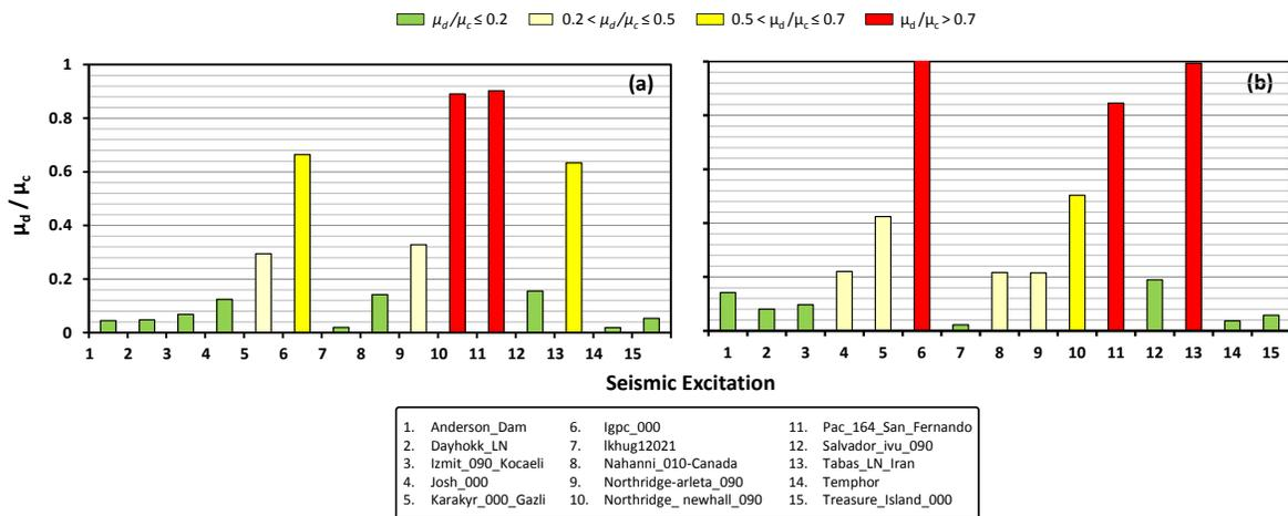
Figure 5. Comparison of (a) observed damage states based on ductility demand over ductility capacity  $\mu_d/\mu_c$  of the FE analysis with (b) predicted ones based on the proposed nonlinear regression model equation for 15 historic out-of-sample records, and differences between them.
