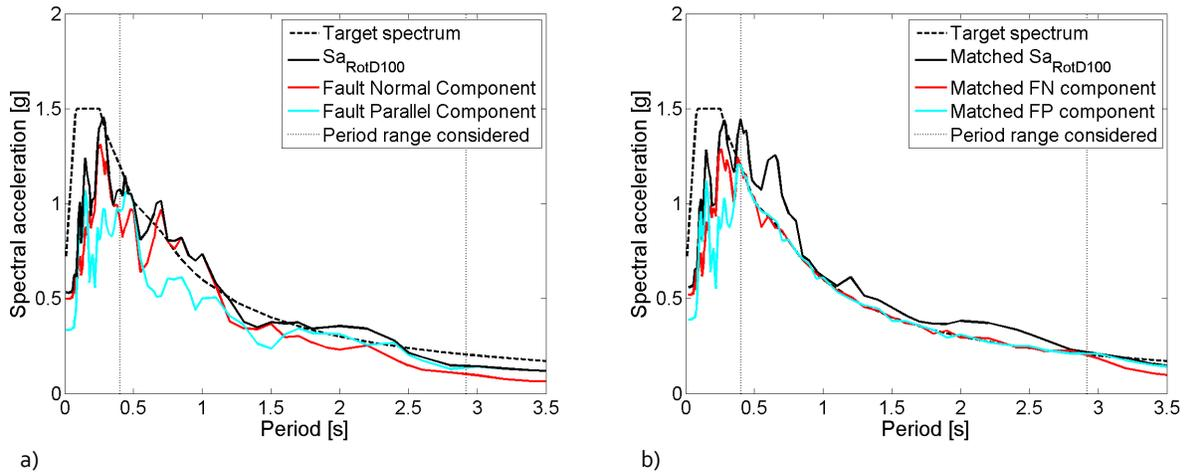
Figure 2: Response spectra of a single ground motion, (a) before and (b) after spectral matching. The ground motion is the West 15<sup>th</sup> Street recording from the 1994 Northridge earthquake.
