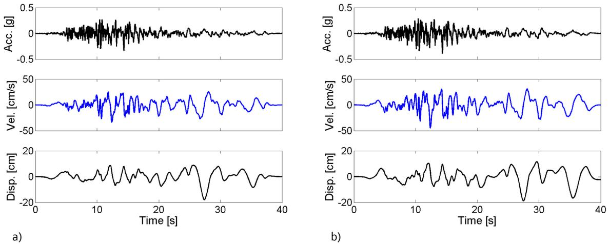
Figure 3: The Fault Normal component of the West 15<sup>th</sup> Street recording from the 1994 Northridge earthquake, (a) before and (b) after spectral matching.
