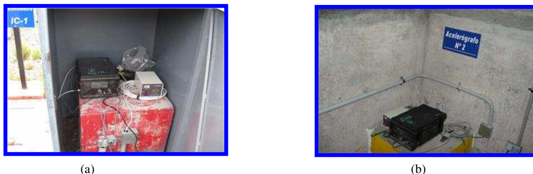
Figure 1. Accelerometers installed in the dam (a) Accelerometer installed at the crest dam. (b) Accelerometer installed at the bedrock level
