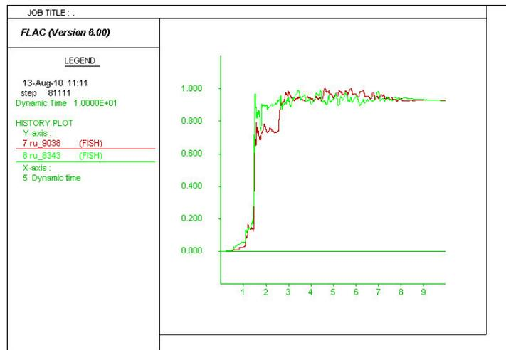
**Figure 11. Traces of excess pore pressure ratios (Westmoreland Fire Station, 1979 Imperial Valley Earthquake)**
