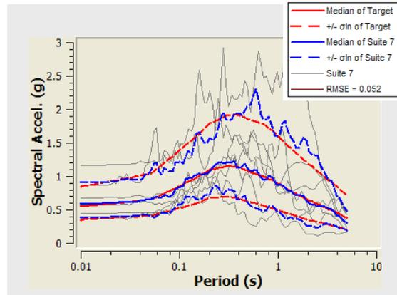
Figure 5. Response Spectra Median  $\sigma_n$  of Suite of 7 Ground Motions
