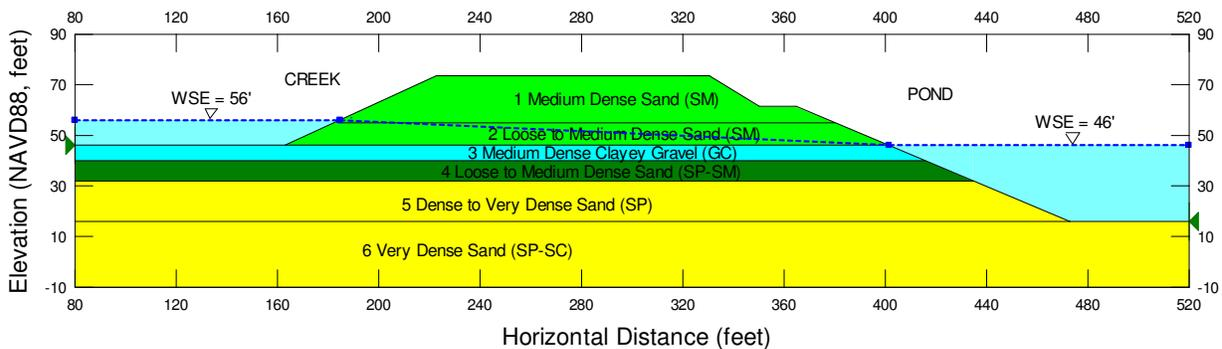
**Figure 3. The generalized cross section**
