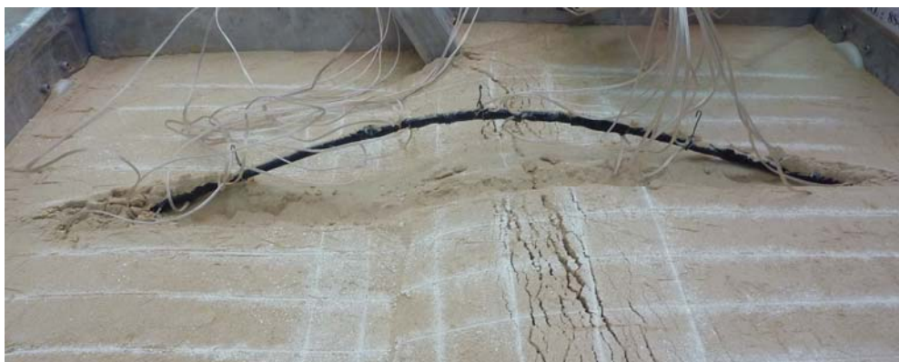
Figure 7. Surface Observation of 2 nd test (Beam buckling of pipe due to reverse faulting)
