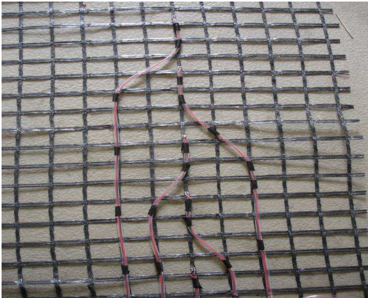
Fig. 4. Strain gage setup on geogrid
