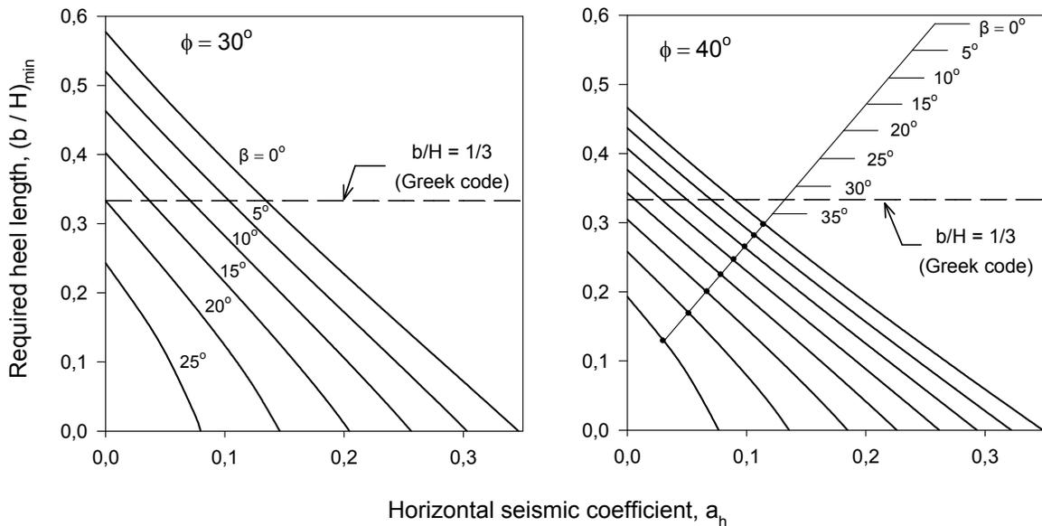
**Figure 5. Variation of minimum required heel length with horizontal acceleration coefficient and backfill angle.**
