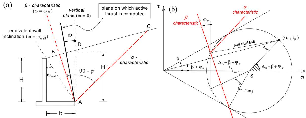
**Figure 4. (a) Rankine wedge in the backfill and applicability condition of Rankine solution, (b) Stress tensor and stress characteristics in the retained soil.**
