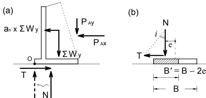
**Figure 8. (a) Equilibrium of forces; (b) equivalent centrically loaded footing according to Meyerhof**
