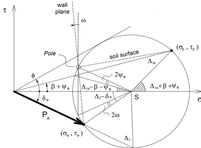
Figure 3 Generalized Rankine stress tensor for earthquake loading
