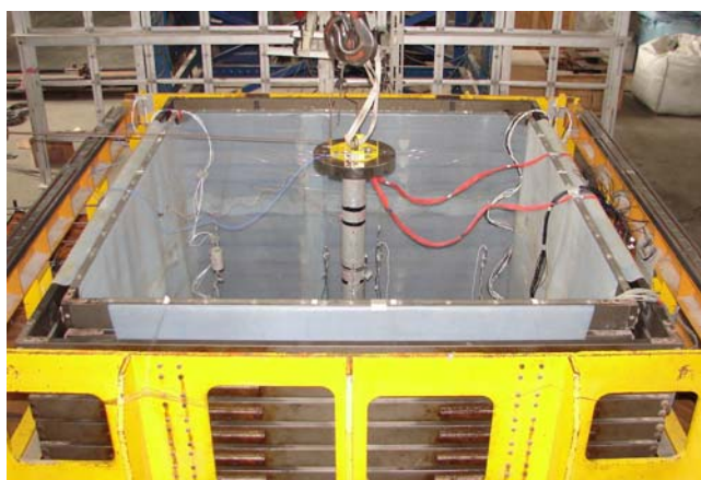
Figure 1. The instrumented aluminum pipe inside the shear box with one steel disk of mass on its top
