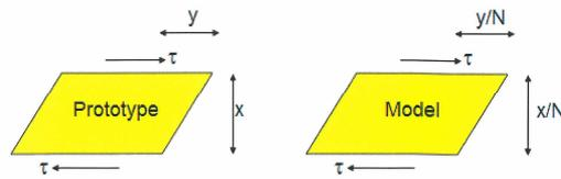
Figure 9. Shear Strain in Prototype and Model Units.
