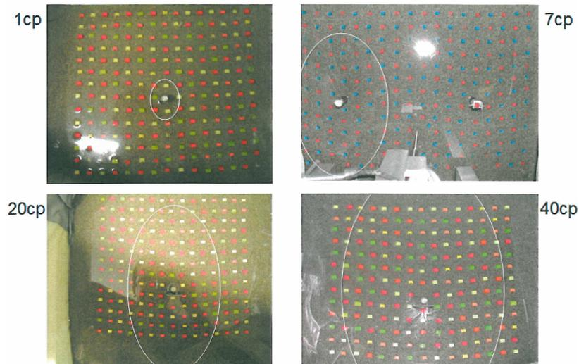
**Figure 5. Soil Deformation around the Pile.**
