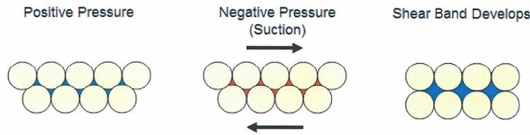
Figure 8. Pore Pressure and Shear Band Development.
