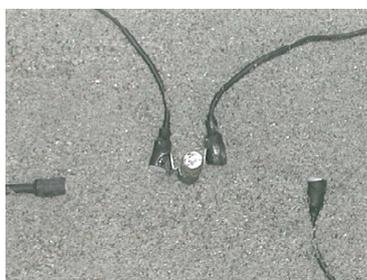
Figure 2. Pore Pressure Transducers around the Pile.
