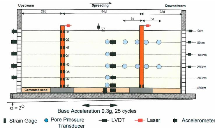
**Figure 1. Centrifuge Models Setup**
