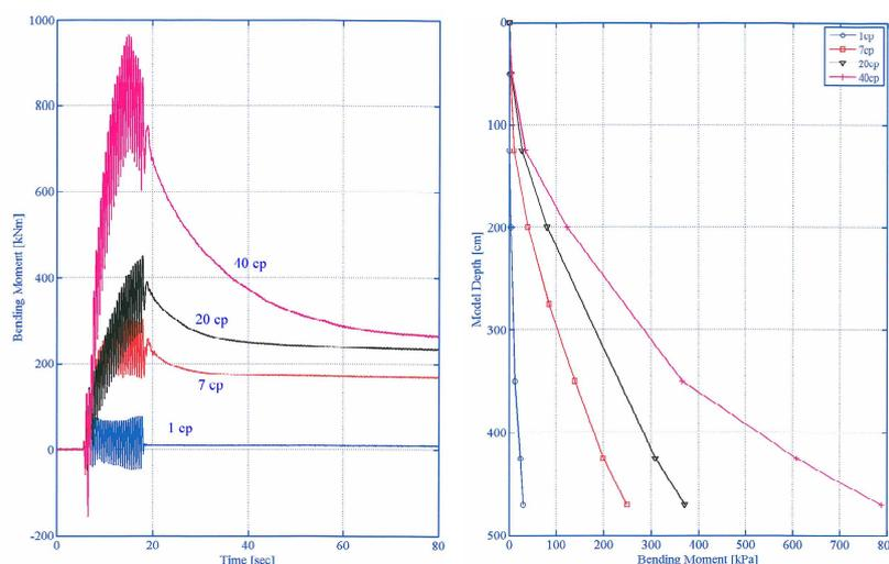
Figure 3. Pile Bending Moments.
