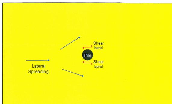
**Figure 7. Schematic Shear Band Development.**
