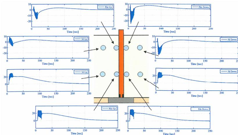
**Figure 4. Excess of Pore Pressure in [kPa] Around the Pile.**
