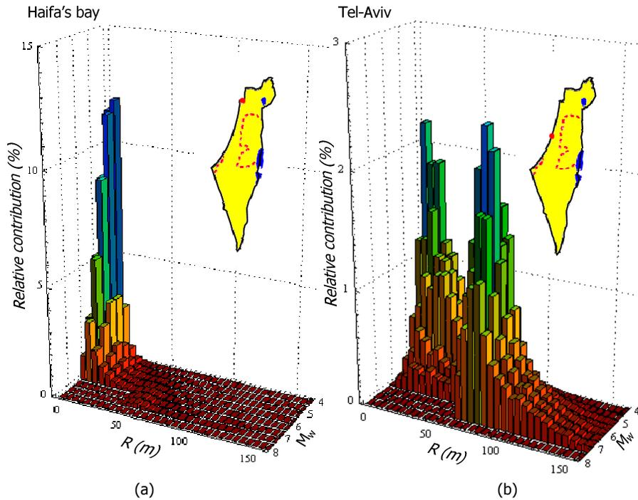
Figure 2. Disaggregation of PGA value at (a) Haifa (PGA=0.23g) and (b) Tel-Aviv (PGA=0.11)
