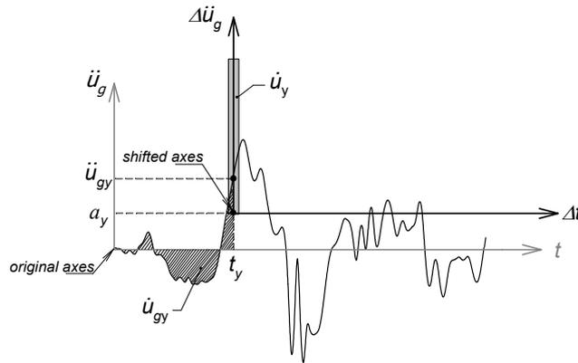
**Figure 3. Translation of axes for an elastic-perfectly plastic system. Shaded areas correspond to initial conditions at yielding.**
