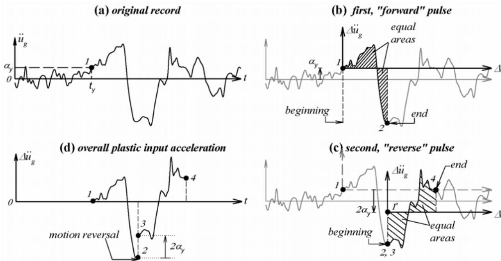
Figure 6. Definition of integration limits and *PIM* according to the proposed approach.
