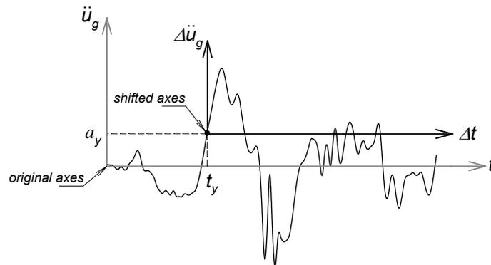
Figure 2. Translation of axes for a rigid – perfectly plastic system.
