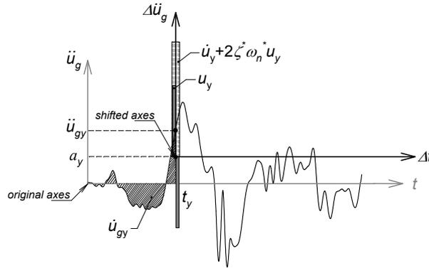
**Figure 4. Translation of axes for a bilinear yielding system. Shaded areas correspond to initial conditions at yielding.**
