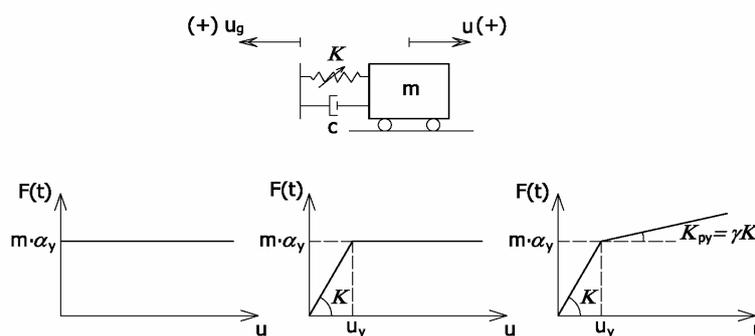
Figure 1. Idealized yielding systems considered in this study. From left to right: (a) Rigid-perfectly plastic, (b) Elastic – perfectly plastic, (c) Bilinear.
