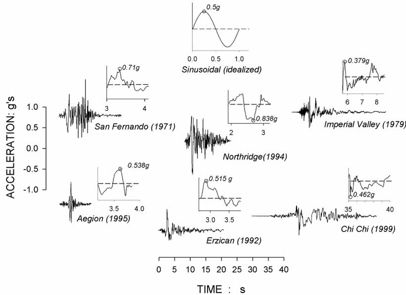
**Figure 5. Selected near-field recorded and idealized ground motions containing long-period, high-acceleration pulses.**
