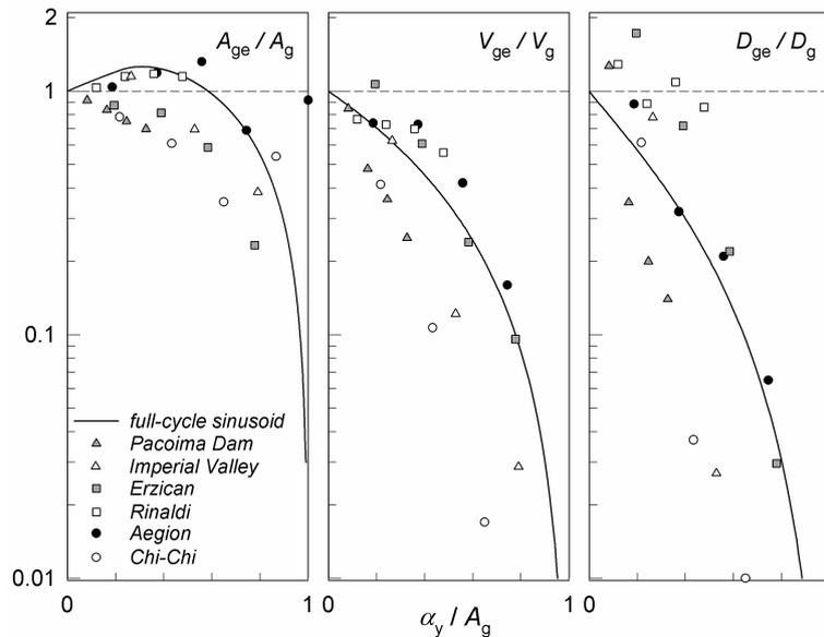
**Figure 10. Peak plastic input motion parameters for the waveforms of Fig 5.**
