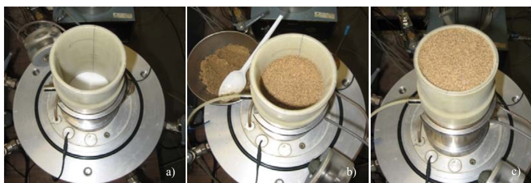
Figure 1. Stages of the assembly: a) fitting the membrane in the mold , b) introducing a layer of sand, c) compaction of the final layer sand in the mold
