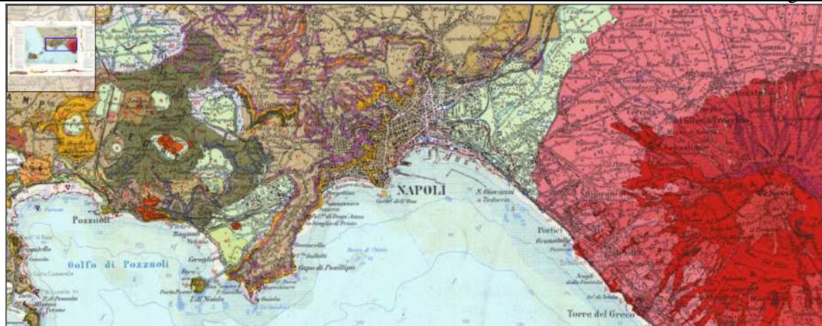
Figure 1. Geological setting of the city of Naples (red: recent lava flow; light green: coastal plan deposits; okra: pyroclastic soils) ( http://www.apat.gov.it/Media/carta_geologica_italia/tavoletta.asp?foglio=183-184 ).
