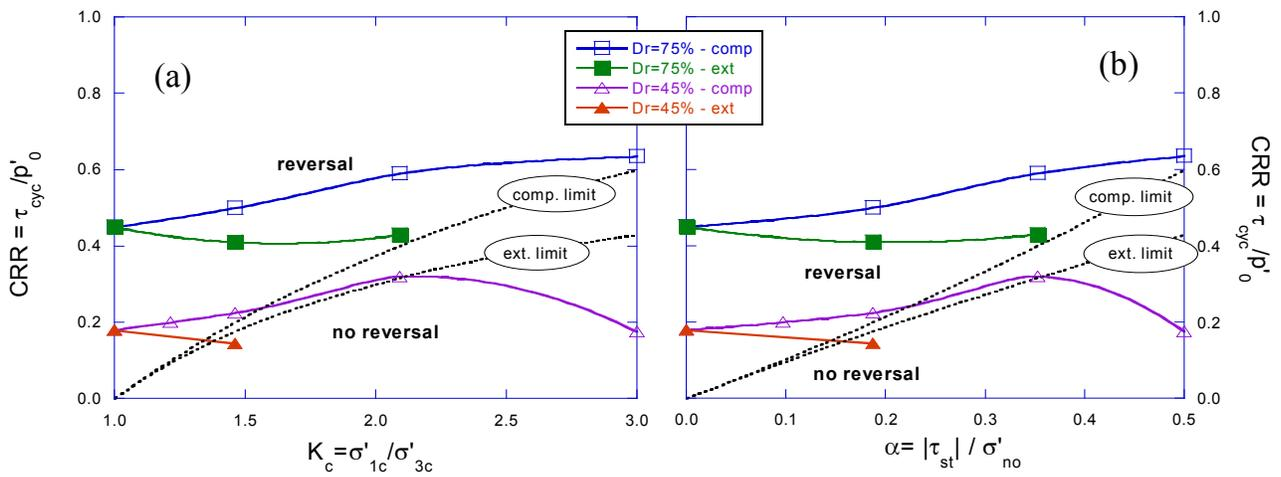
Figure 4. Cyclic Resistance Ratios for  $N=20$ , showing Reverse Load Limits, vs. (a)  $K_c$  and (b)  $\alpha$
