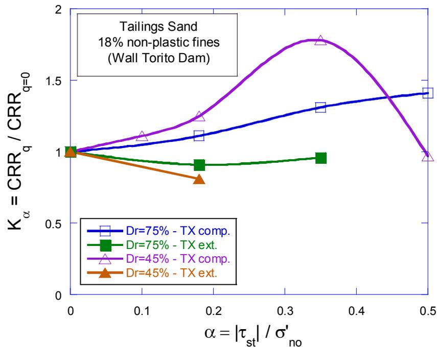
**Figure 5.  $K_\alpha$  vs.  $\alpha$  for Loose and Dense Cases for  $N=20$  and when 5% of D.A. of  $\epsilon_{axial}$  is reached.**
