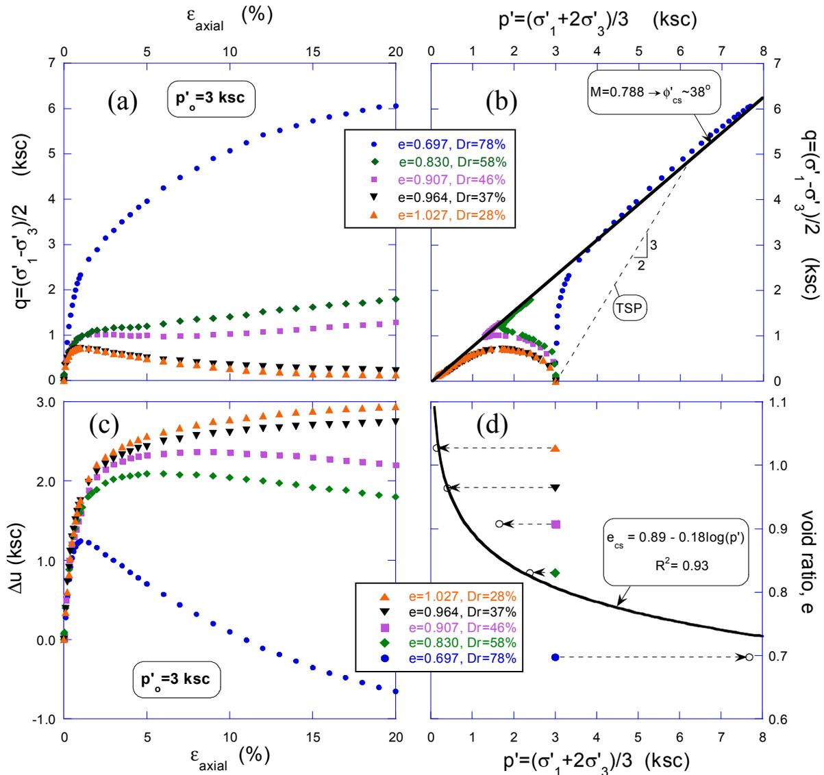
Figure 2. Undrained Triaxial Tests in Compression: (a) Stress-Strain Curves, (b) Effective Stress Paths, (c) Pore Pressure Change and (d) Void Ratio vs. Mean Effective Stress
