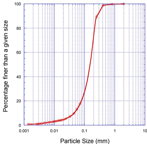
**Figure 1. Granulometric Analysis for Tailings Sand of the Wall Torito Dam**
