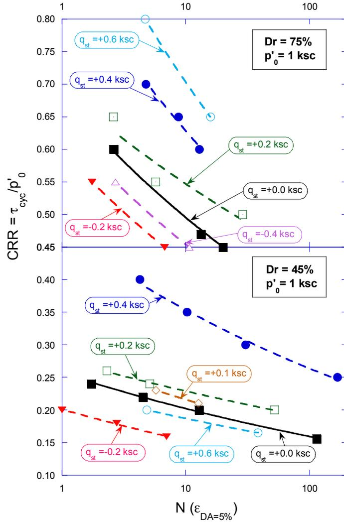
Figure 3. Cyclic Resistance Ratio vs. Number of Cycles to reach 5% of Double Amplitude of  $\epsilon_{axial}$
