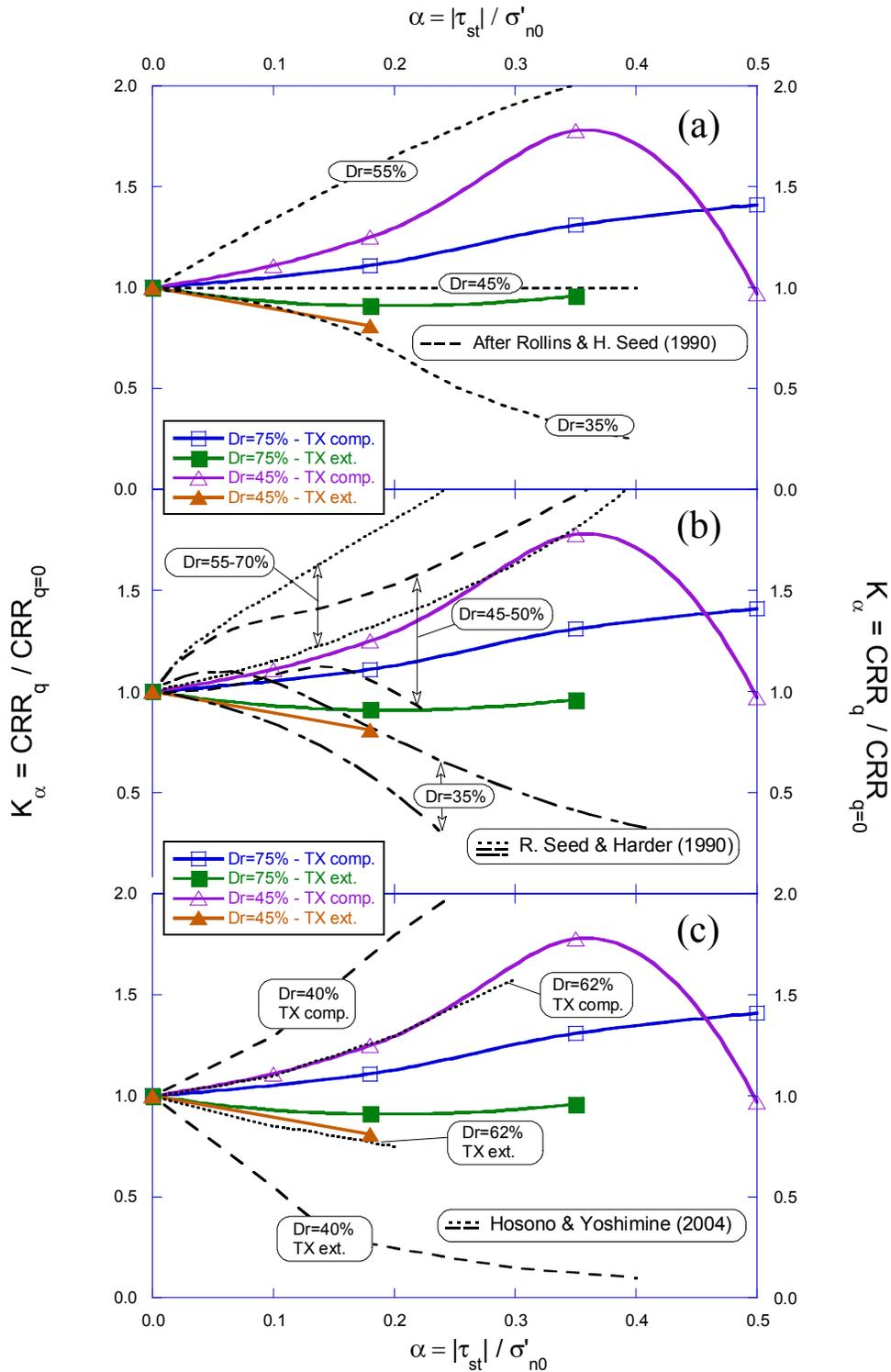
Figure 6: Current Results Compared with (a) Rolling and H. Seed, 1990; (b) R. Seed and Harder, 1990; (c) Hosono and Yoshimine, 2004.
