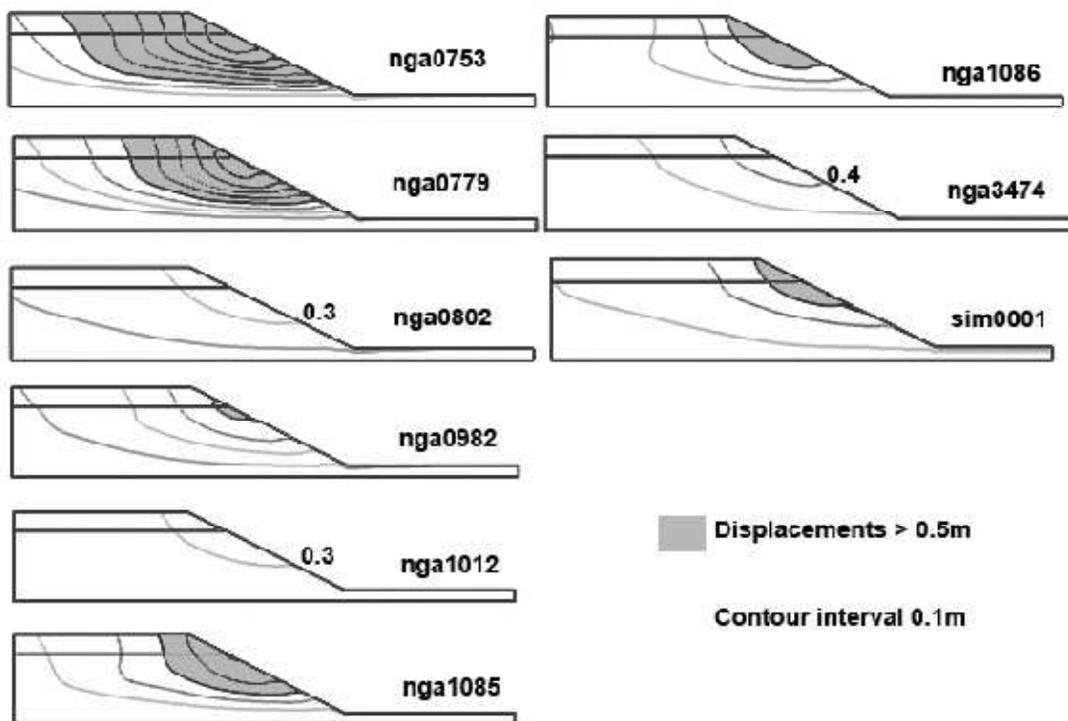
Figure 5. Final deformed shape at end of shaking
