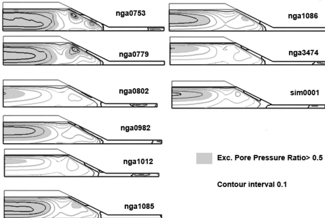
**Figure 6. Excess pore pressure ratios at the end of the strong ground motion**
