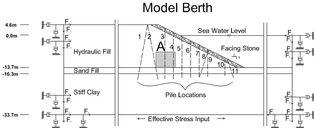
Figure 1 Modeled geometry; region A defines a region used subsequently in the averaging of excess pore pressures to define excess pore pressure vs damage correlations
