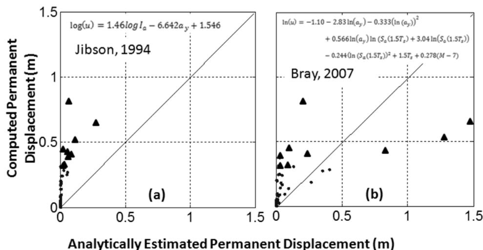
**Figure 4 Comparison of the displacement on top of the slope (y-axis) with slope displacements from analytical correlations (x-axis), triangles indicate motions that cause large damage; (a) Jibson (1994) (b) Bray (2007)**
