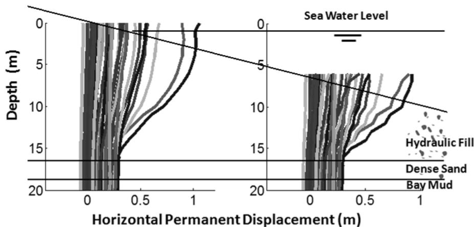
**Figure 7 Final horizontal displacements along two sections where piles are installed for all the ground motions. Each line represents the final horizontal deformation profile for each motion**
