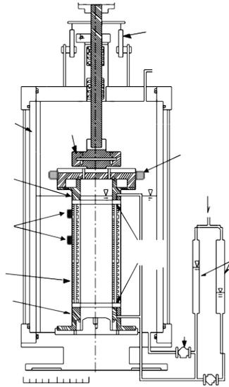
Figure 1. Torsional shear apparatus
