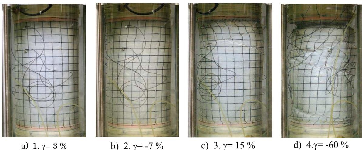
**Photo 1. Specimen deformation at status 1 through 4 in Fig. 5**
