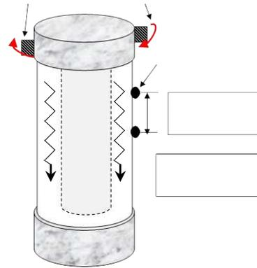
Figure 2. Diagram of S wave triggers and accelerometers on a hollow cylindrical specimen
