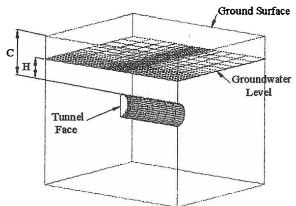
Figure 3. 3-Dimensional condition for seepage analysis.
