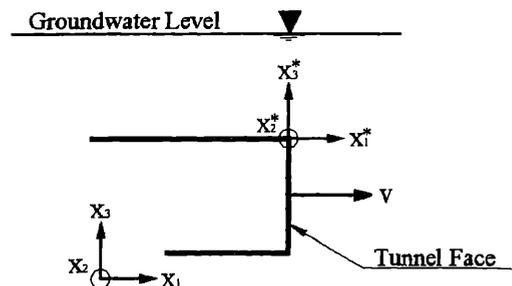
Figure 6. Concept of face-fixed frame of reference.
