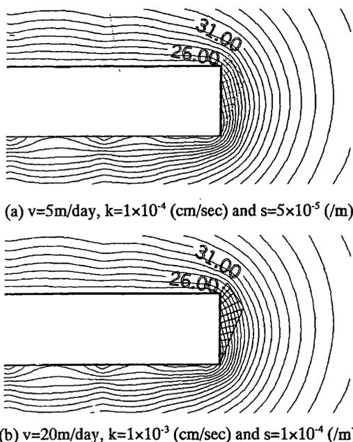
Figure 7. Hydraulic head distributions around the tunnel ( $Dsv/k=0.014$  in both cases).
