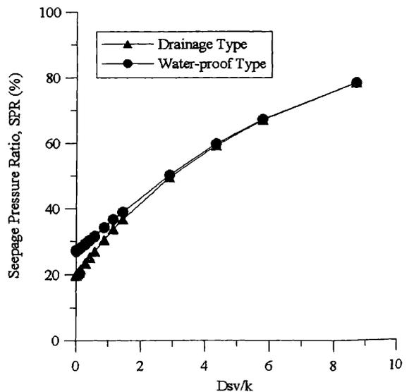
Figure 8. Dimensionless parameter  $Dsv/k$  - seepage pressure ratio (SPR) relationship.
