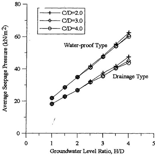
Figure 4. Average seepage pressure with the variation of the H/D ratio.
