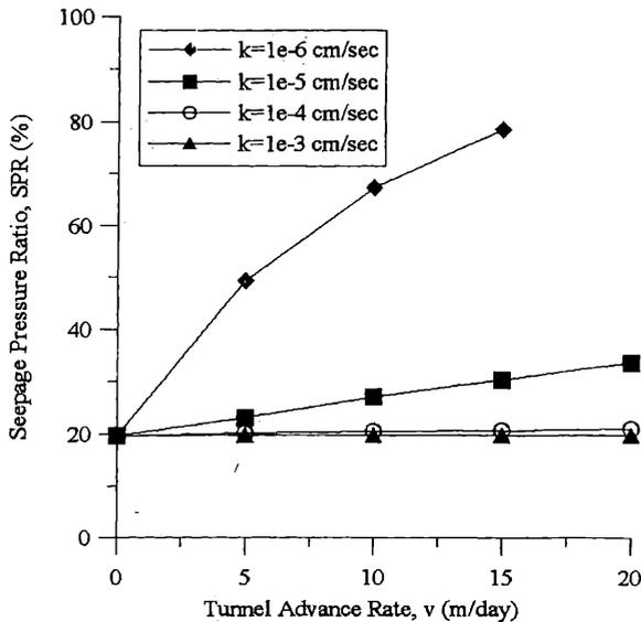
Figure 9. Tunnel advance rate ( $v$ ) - seepage pressure ratio (SPR) relationships (In case of  $s=1 \times 10^{-4}$ /m).
