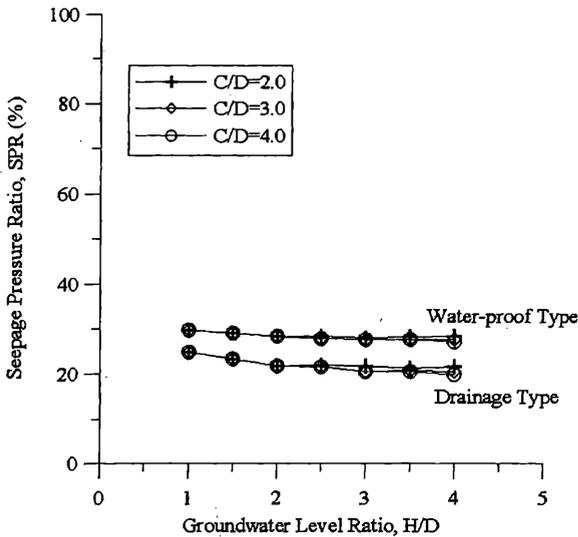
Figure 5. Seepage pressure ratio with the variation of the H/D ratio.
