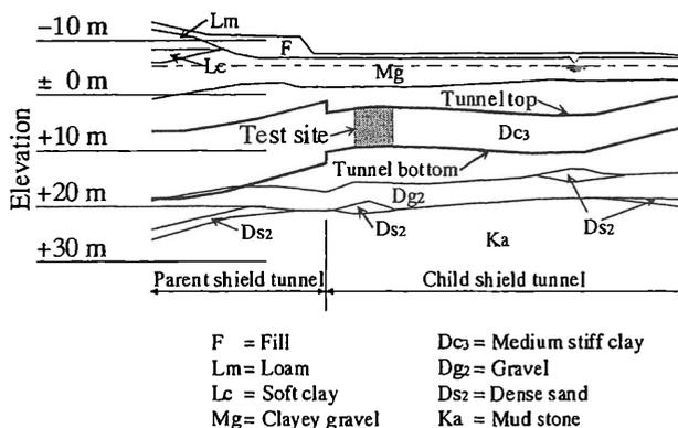
Figure 1. Geological profile at test site location.
