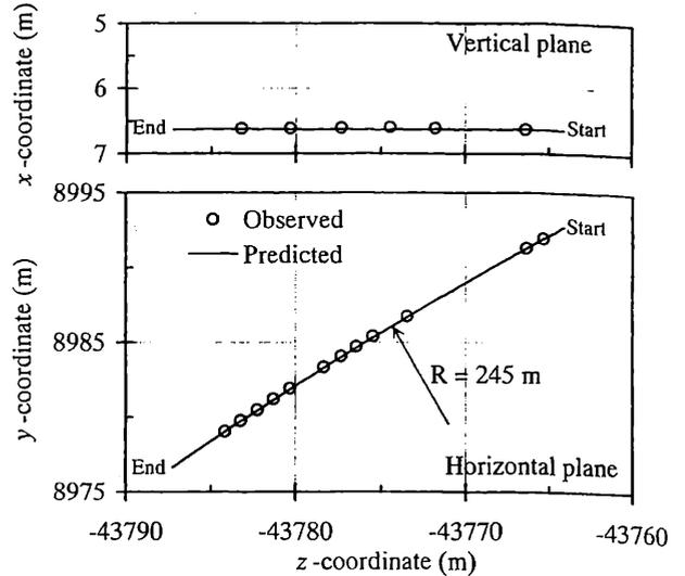
Figure 6. Predicted and observed shield traces.
