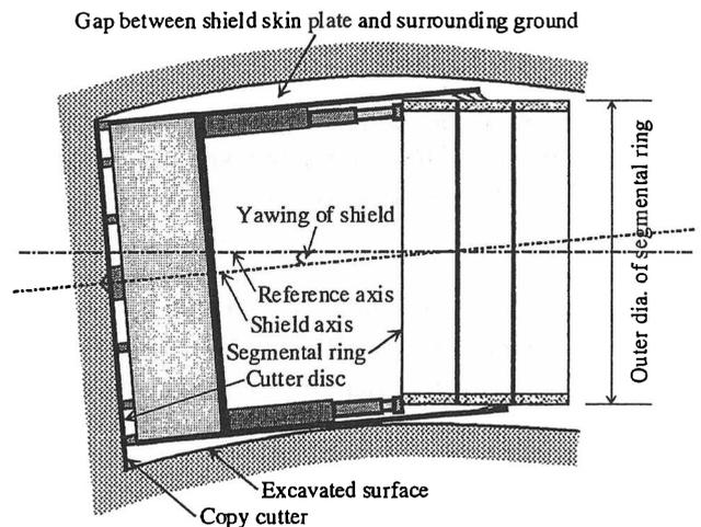
Figure 9. Illustration of gap around shield during excavation.
