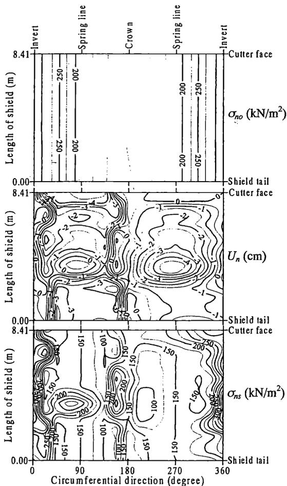
Figure 7.  $\sigma_n$  and  $U_n$  around shield at distance of 150.011 m.
