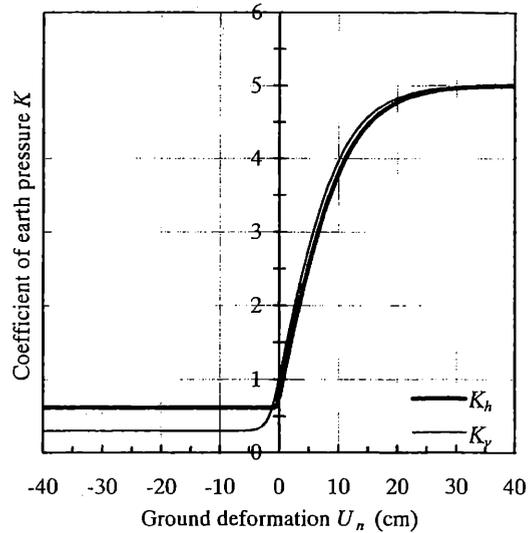
Figure 8. Ground reaction curves for medium stiff clay layer.
