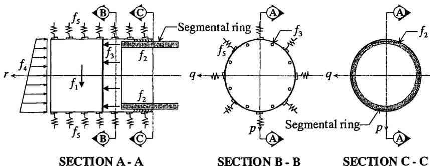
Figure 4. Model of loads acting on shield.
